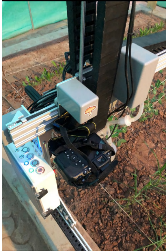
Figure 3. Camera mounted over Farmbot
