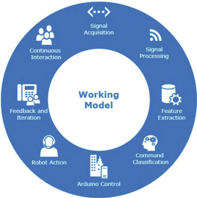
FIGURE 14.2 Working model of the brain-controlled Arduino robot.
