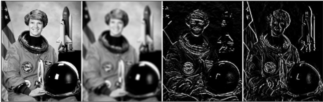
Figure 4.4 – The first image is the grayscale input. The second image is the result of a 10 \times 10 blur filter. The third and fourth images use detectors and vertical Sobel edge detectors
