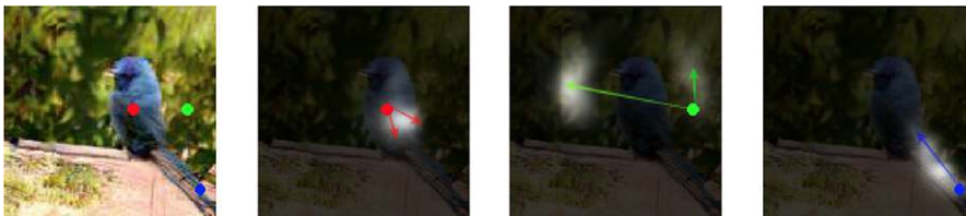
Figure 10-16. A SAGAN-generated image of a bird (leftmost cell) and the attention maps of the final attention-based generator layer for the pixels covered by the three colored dots (rightmost cells) (source: Zhang et al., 2018)
