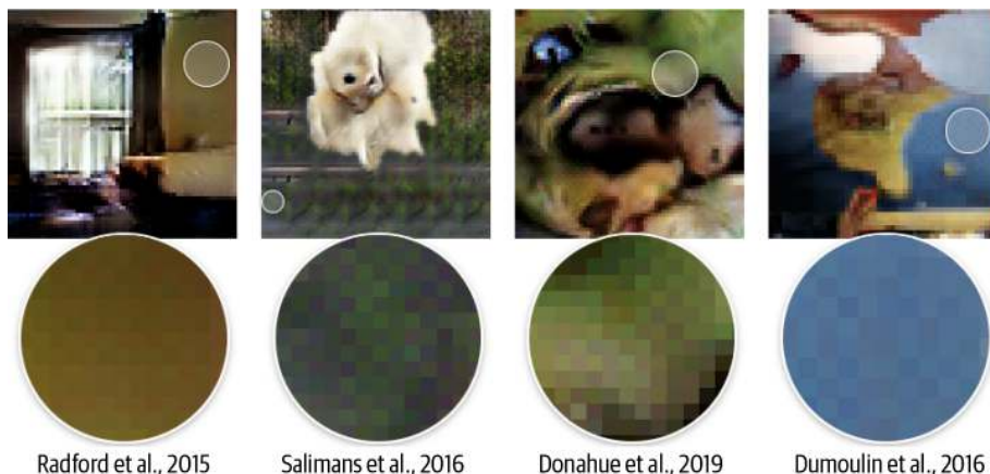
Figure 4-4. Artifacts when using convolutional transpose layers (source: Odena et al., 2016 ) 3
