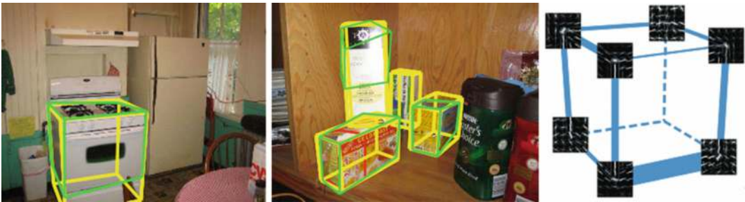
Fig. 7.4 Annotated or labeled ground truth dataset images for scene analysis of cuboids (left and center). The labels are annotated manually into the ground truth dataset, in yellow (light gray in B&W version) marking the cuboid edges and corners. (Right) Ground truth data contains precomputed 3D corner HOG descriptor sets, which are matched against live detected cuboid HOG feature sets. Successful matches shown in green (dark gray in B&W version). (Images used by permission © Bryan Russel, Jianxiong Xiao, and Antonio Torralba)
