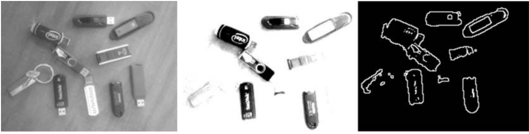
Fig. 2.4 Use of thresholding to solve problems during image preprocessing to prepare images for polygon shape measurement: (Left) Original image. (Center) Thresholded red channel image. (Right) Perimeter tracing above a threshold
