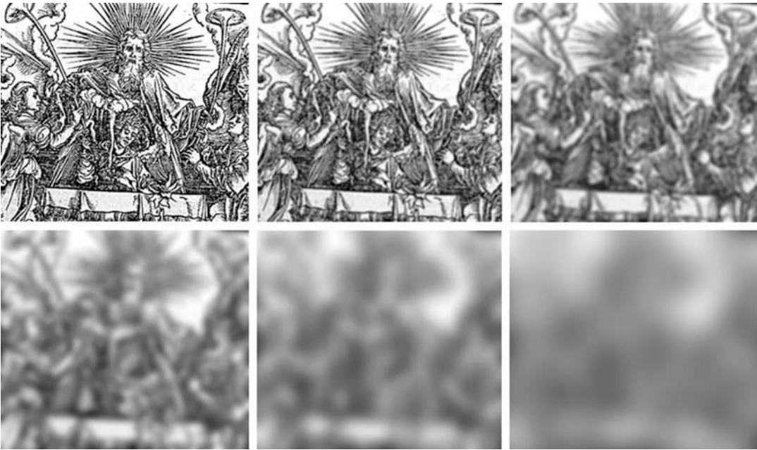
Fig. 4.17 Scale space Gaussian images at scales of 0, 2, 4, 16, 32, 64. (Image is from Albrecht Durer's Apocalypse woodcuts, 1498)
