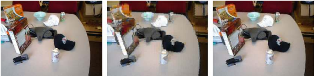
Fig. 10.75 This figure illustrates image reconstruction from sparse codes, each codeword is a 5 \times 5 image patch. (Left) original, (center) reconstruction using two codewords and looking blocky, (right) reconstruction using five codewords and working well. Image from Bo et al. [204] from ISER Springer Tracts in Advanced Robotics, © Springer used by permission
