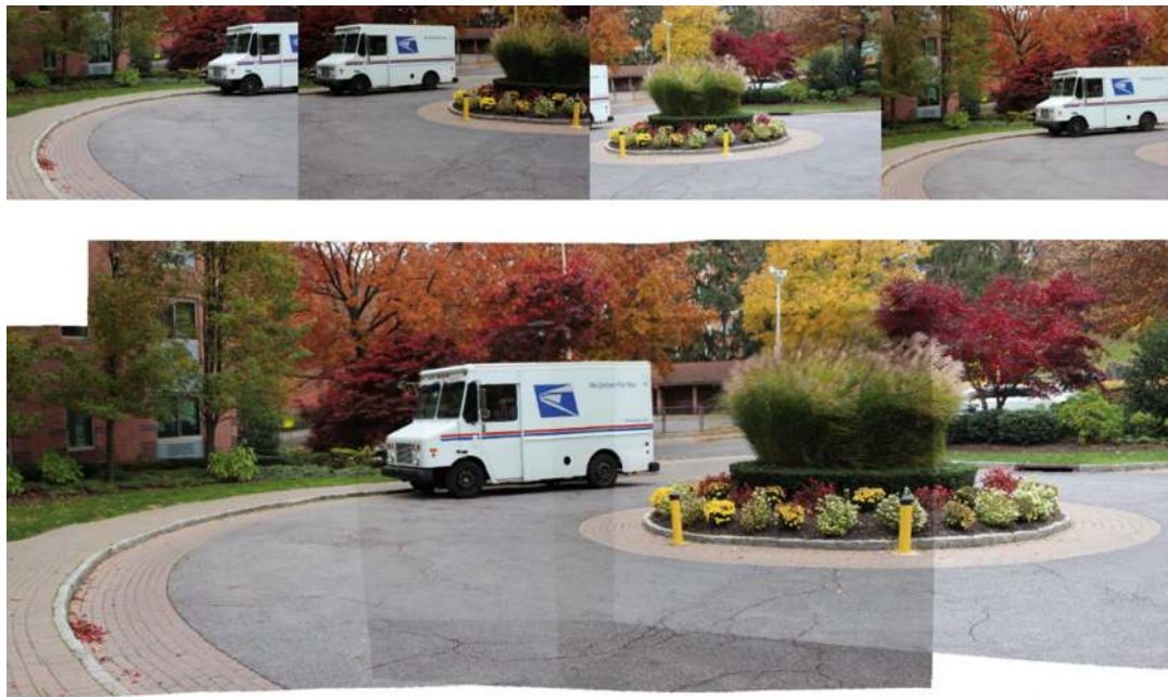
Fig. 12.8 Results of the Adaptive 2D Image Stitching method, showing (top) original unstitched images and (bottom) final stitched image, images published at CVPR 2015 (C) 2015 Ching Lin et al. [866], used by permission from Springer Verlag
