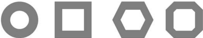
Fig. 6.19 CenSurE bilevel center-surround filter shape approximations to the Laplacian using binary kernel values of 1 and -1 , which can be efficiently implemented using signed addition rather than multiplication. Note that the circular shape is the desired shape, but the other shapes are easier to compute using integral images, especially the rectangular method
