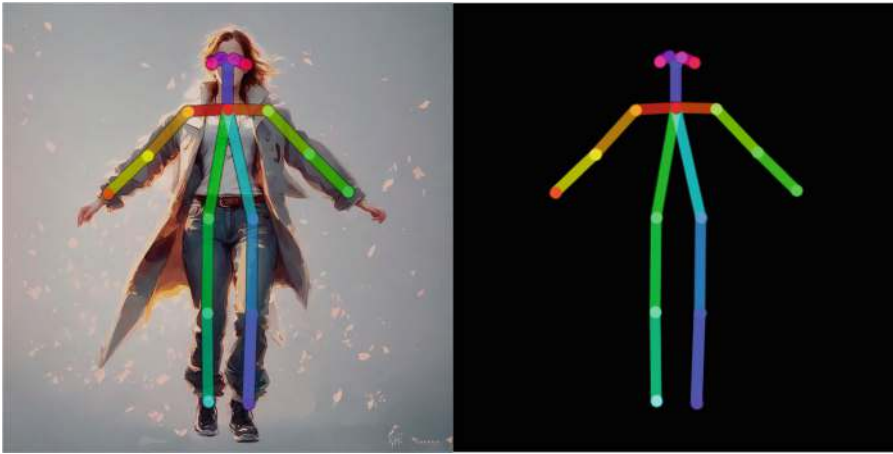
Fig. 8.6 Pose points for human body joints created using the Openpose method analyzing synthetic diffusion model images using view synthesis, images courtesy of openposes.com —images available for public use—© Openposes.com . There are many methods available for pose points, including 3D and 6DOF
