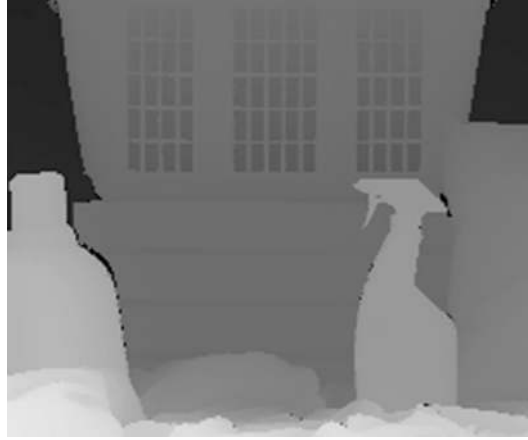
Fig. 4.19 Segmentation of image regions based on a depth map. Depth image from Middlebury Data set. (Source: D. Scharstein and C. Pal “Learning conditional random fields for stereo” CVPR Conference, 2007. Courtesy of authors)
