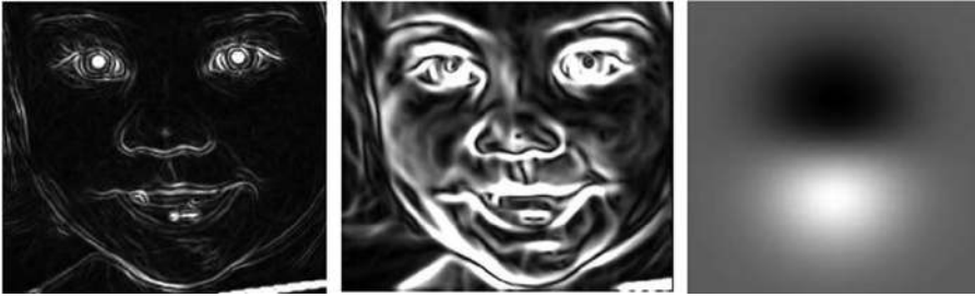
Fig. 8.8 Location of facial landmarks. (Left) Facial landmarks enhanced using largest eigenvalues of Hessian tensor [420] in FeatureJ; note the fine edges that provide extra detail. (Center) Template-based feature detector using steerable filters with additional filtering along the lines of the Canny detector [331] to provide coarse detail. (Right) Steerable filter pattern used to compute center image. Both images are enhanced using contrast window remapping to highlight the edges. FeatureJ plug-in for ImageJ used to generate eigenvalues of Hessian (FeatureJ developed by Erik Meijering)
