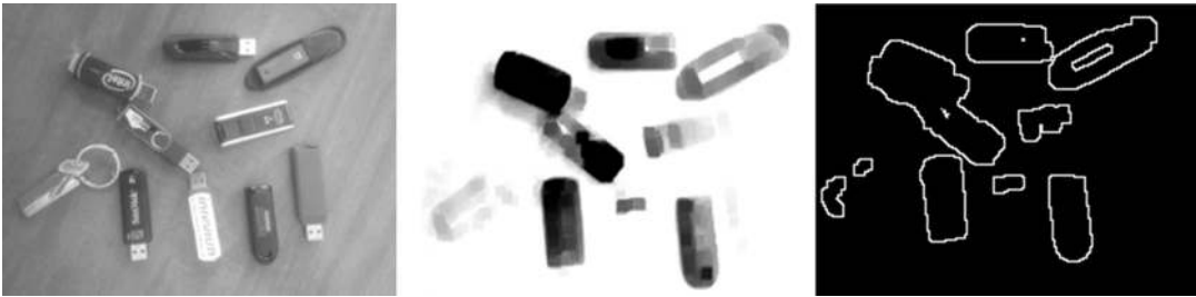
Fig. 2.5 Another sequence of morphological preprocessing steps preceding polygon shape measurement: (Left) Original image. (Center) Range thresholded and dilated red color channel. (Right) Morphological perimeter shapes taken above a threshold
