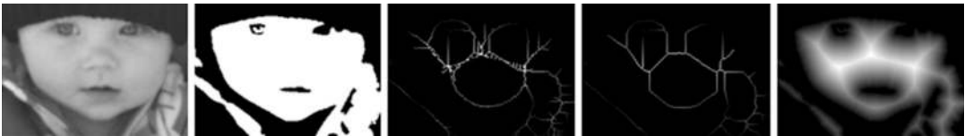
Fig. 6.5 Morphological methods to find interest regions. (Left to right) Original image, binary thresholded, and segmented image using Chan-Vese method, skeleton transform, pruned skeleton transform, and distance transform image. Note that binary thresholding requires quite a bit of work to set parameters correctly for a given application
