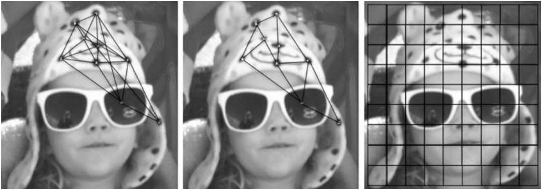
Fig. 4.7 Reduced resolution examples of the D-NETS [106] sampling patterns. (Left) Full dense connectivity at interest points. (Center) Sparse connectivity at interest points. (Right) Dense connectivity over a regular sampling grid. The D-NETS authors note that a dense sampling grid with 10 pixel spacing is preferred over sampling at interest points
