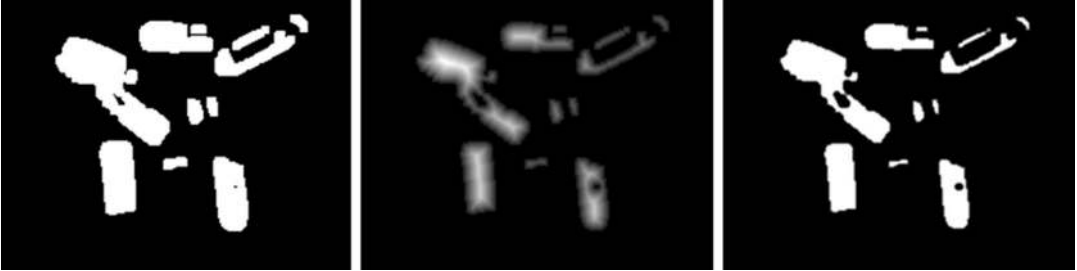
Fig. 2.18 Preprocessing sequence: (Left) Image after thresholding and erosion. (Center) EDM showing gray levels corresponding to distance of pixel to black background. (Right) Simple binary thresholded EDM image
