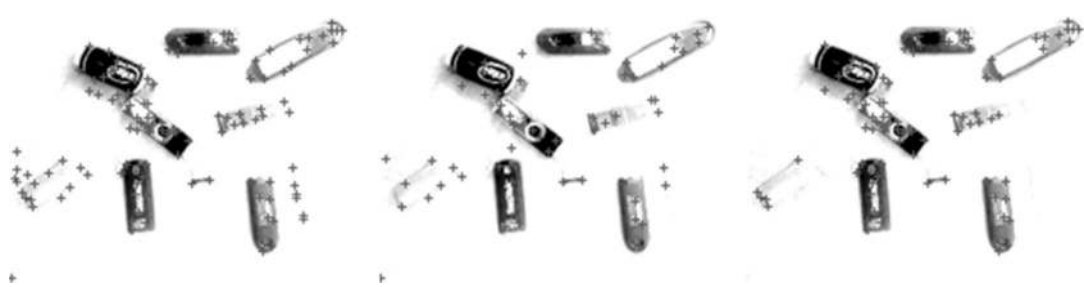
Fig. 7.7 Machine corner detection using the Shi–Tomasi method marked with crosses; results are shown using different parameter settings and thresholds for the strength and pixel size of the corners
