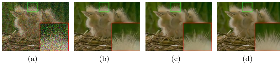
FIGURE 14.3 Color image denoising results of different methods on image “163085” from CBSD68 dataset with noise level 50. (a) Noisy (14.99 dB); (b) DnCNN (28.68 dB); (c) FFDNet (28.75 dB); (d) DRUNet (29.28 dB).
