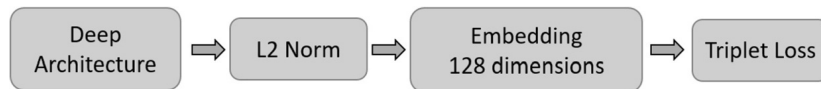
FIGURE 6.7 The general architecture of FaceNet model. A key aspect of the FaceNet model is the ability to classify a given face image using an embedding of 128 deep features.
