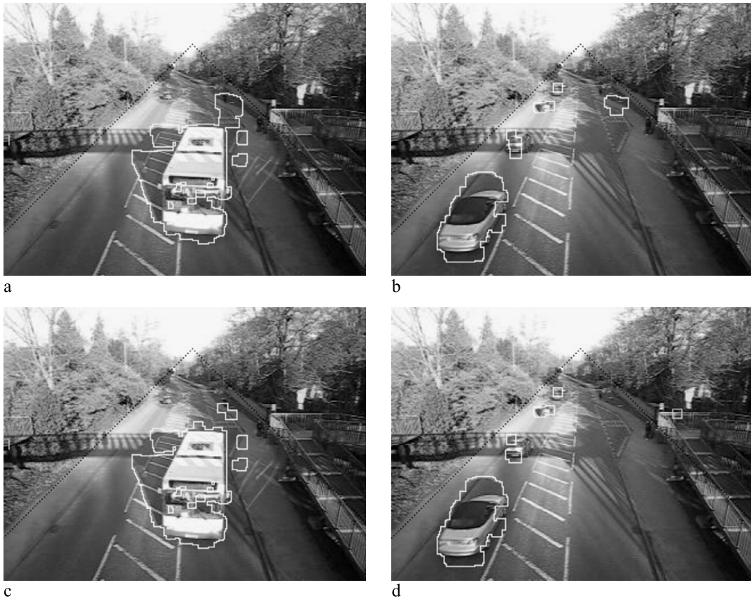
FIGURE 1.27 Background subtraction using a temporal median filter. Note the plethora of stationary shadows that are completely ignored during the process of background subtraction. In (a) the ‘ghost’ of the bus (from its past position) still appears, but in (b) it has started to merge back into the background: the problem is considerably reduced in (c) and (d), which uses a ‘restrained’ temporal median filter. Overall, foreground object fragmentation and false shapes (including the effects of moving shadows) are the worst problems. The lines of black graphics dots demarcate the relevant road region: almost all of the fluttering vegetation lies outside this region.
