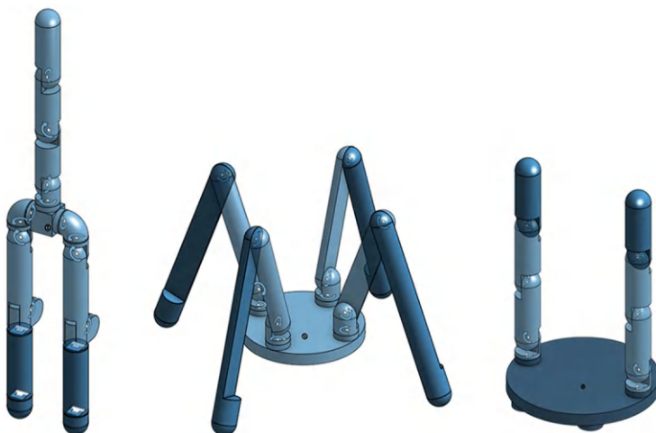
Fig. 12.12 Non-anthropomorphic morphologies. The images depict three different non-anthropomorphic morphologies that are trained to exhibit expressive movements. From left to right: Biped , Quadruped , Legless . The body parts rendered in dark blue have been assigned foot or hand status
