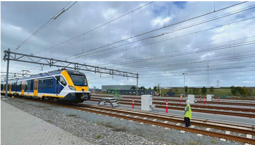
Fig. 5.4 Automatic Train Operation (ATO) is able to detect dummies on the track and stop the train automatically. Image property of CAF
