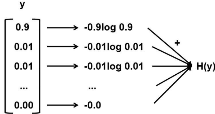
Fig. 4.1 Schematic diagram of entropy calculation
