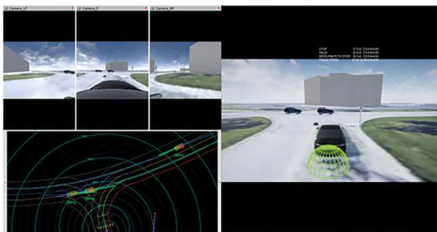
Figure 6.6 Neuromorphic Stanley controller with 2,500 neurons introduces Zig-Zag patterns.
