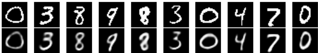
Figure 2.5 – The first row is the input image and the second row is generated by the autoencoder
