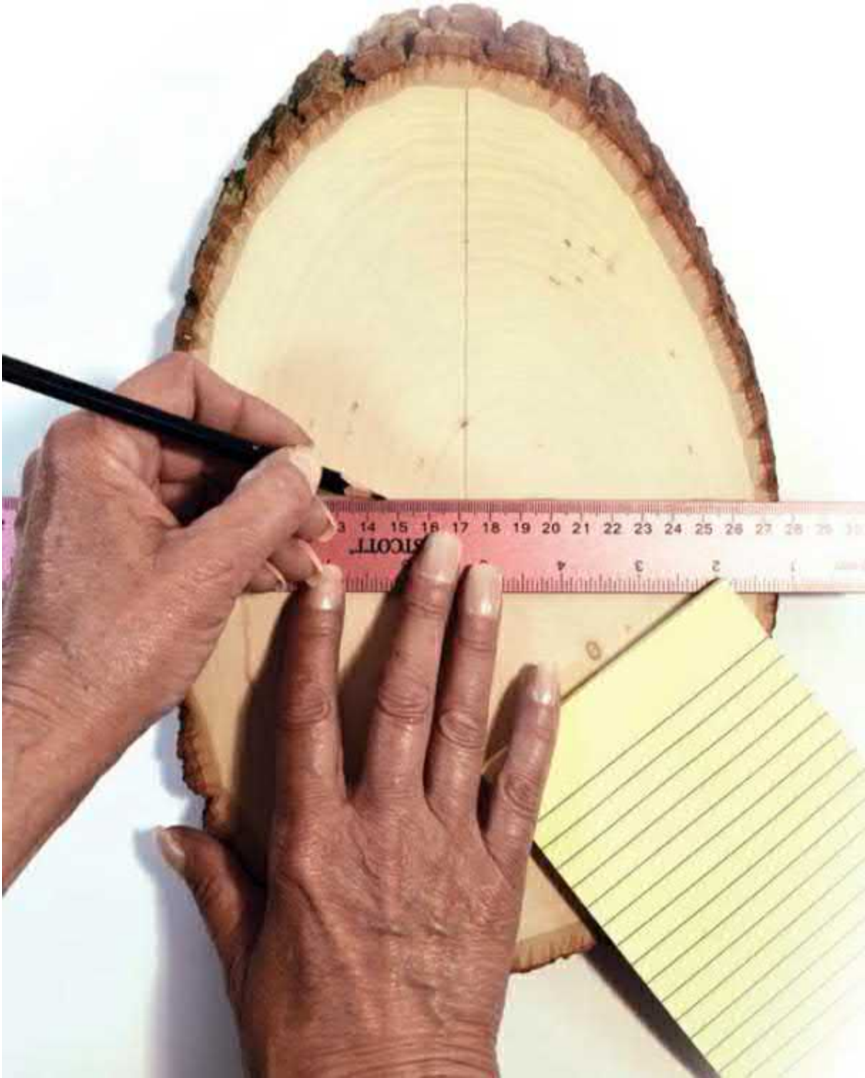
Figure 1.21. Create vertical and horizontal lines with a ruler and other square-edged materials you have at home. Drawing a level line on any surface is made easy by measuring spots on either side of your center point.
