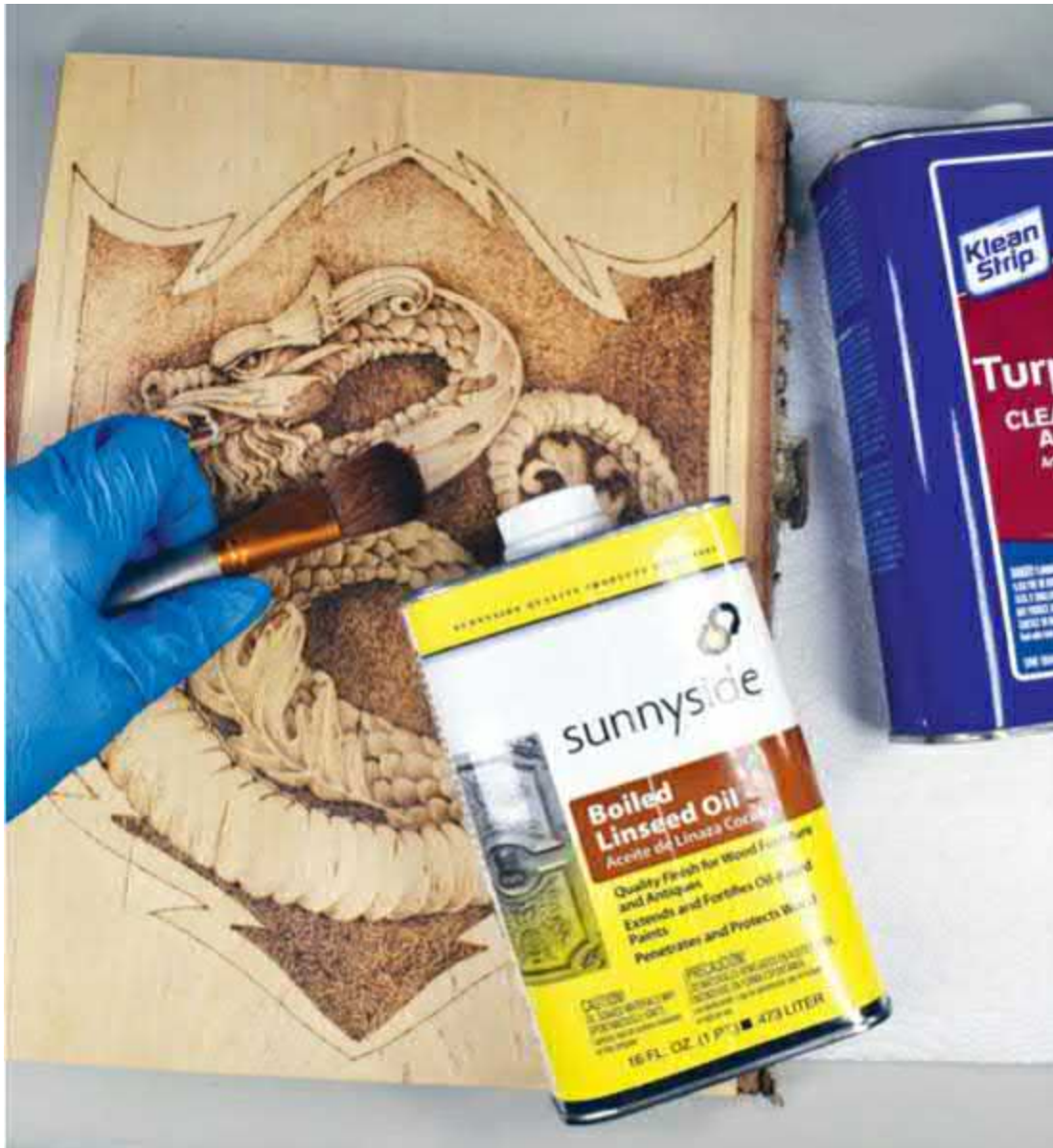
Figure 1.35. Oil finishes are popular because they penetrate the wood to enhance the natural grain. However, this method can sometimes darken pyrography work.
