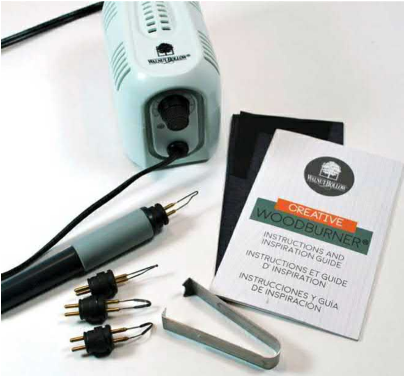
Figure 1.5. For the projects and practice board shown in this book, I use a Walnut Hollow Creative Woodburner. It's a variable-temperature tool with four interchangeable pen tips.
