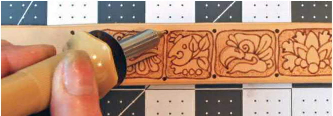
Figure 1.3. A one-temperature tool with a low temperature is perfect for leather and cloth burnings.
