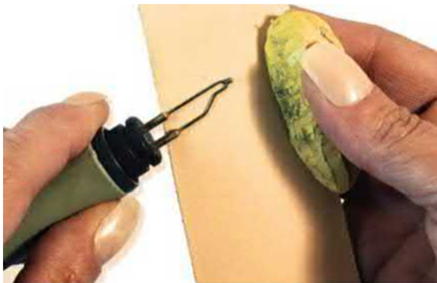
Figure 1.12. Turn your leather scrap over. Working on the tanned-leather side without rouge will brighten the polish on your tip.
