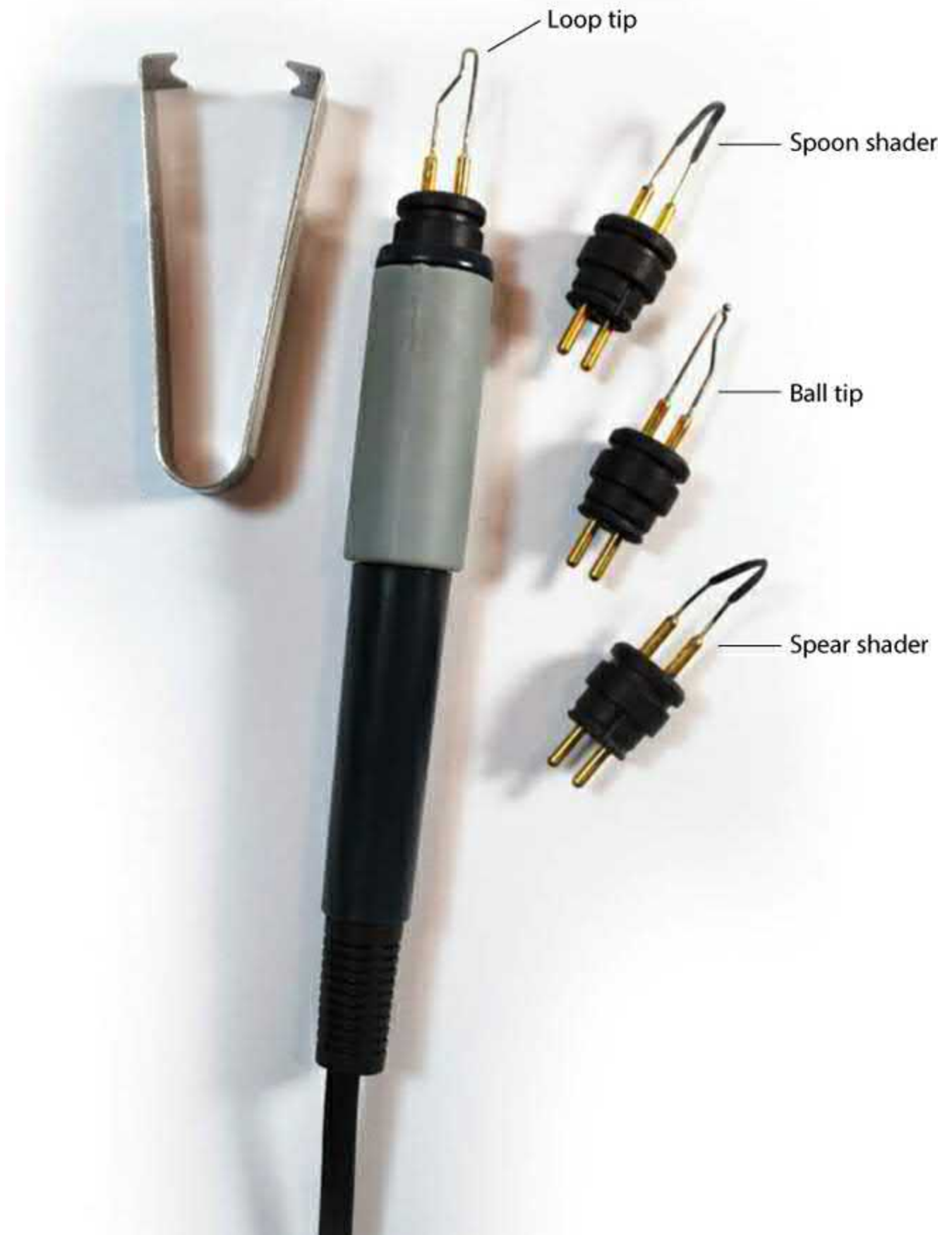
Figure 1.8. Each manufacturer has their own names for the pen tip profiles. In general you will use a loop tip, curved
