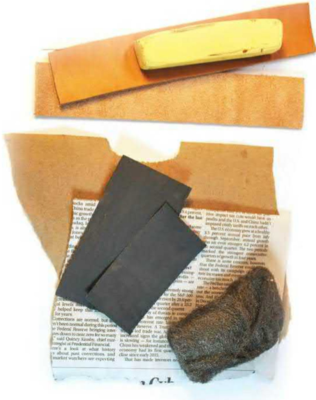
Figure 1.10. Materials needed for cleaning woodburning pen tips. From top to bottom: yellow oxide rouge, tanned leather, raw leather, heavy kraft paper, emery cloth, newspaper, and fine steel wool.
