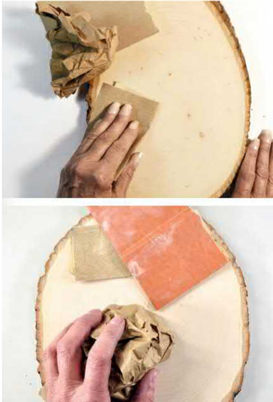
Figure 1.19. The smoother your wood surface, the finer and straighter your detailing lines can be. Always sand with the grain of the wood, using progressively finer-grit papers. End with a good polishing of the wood surface using heavy kraft paper.
