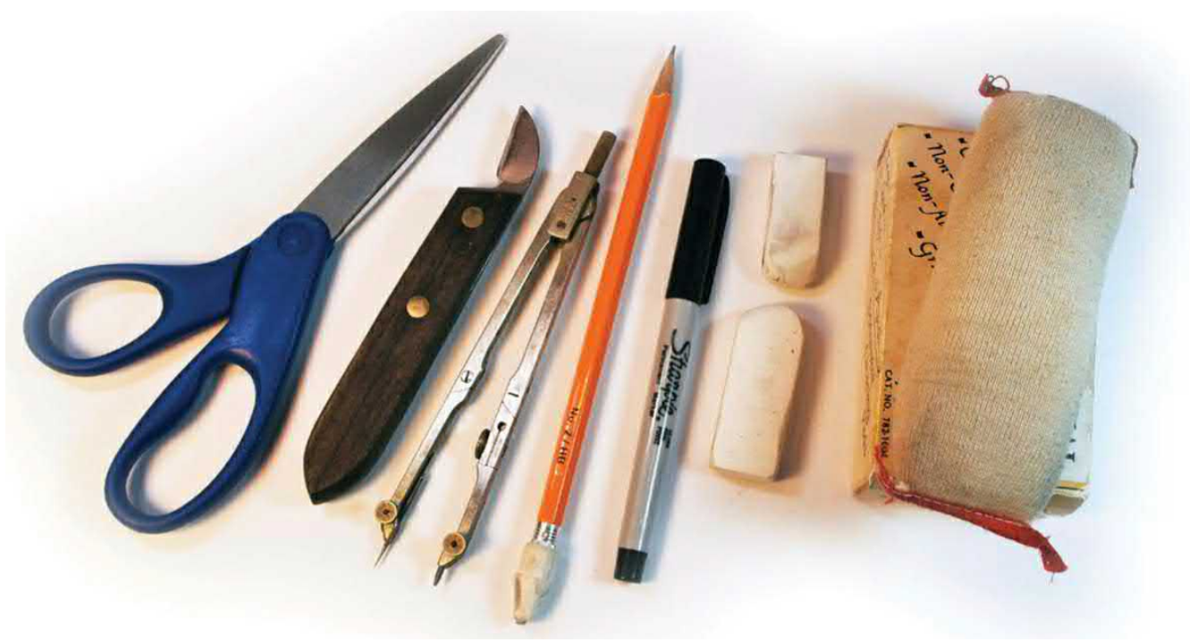
Figure 1.9. Some of the items you'll need. From left to right: scissors, bench knife, compass, #2 or softer graphite pencil, fine-point permanent marking pen, white erasers, and an architect's erasing pad.
