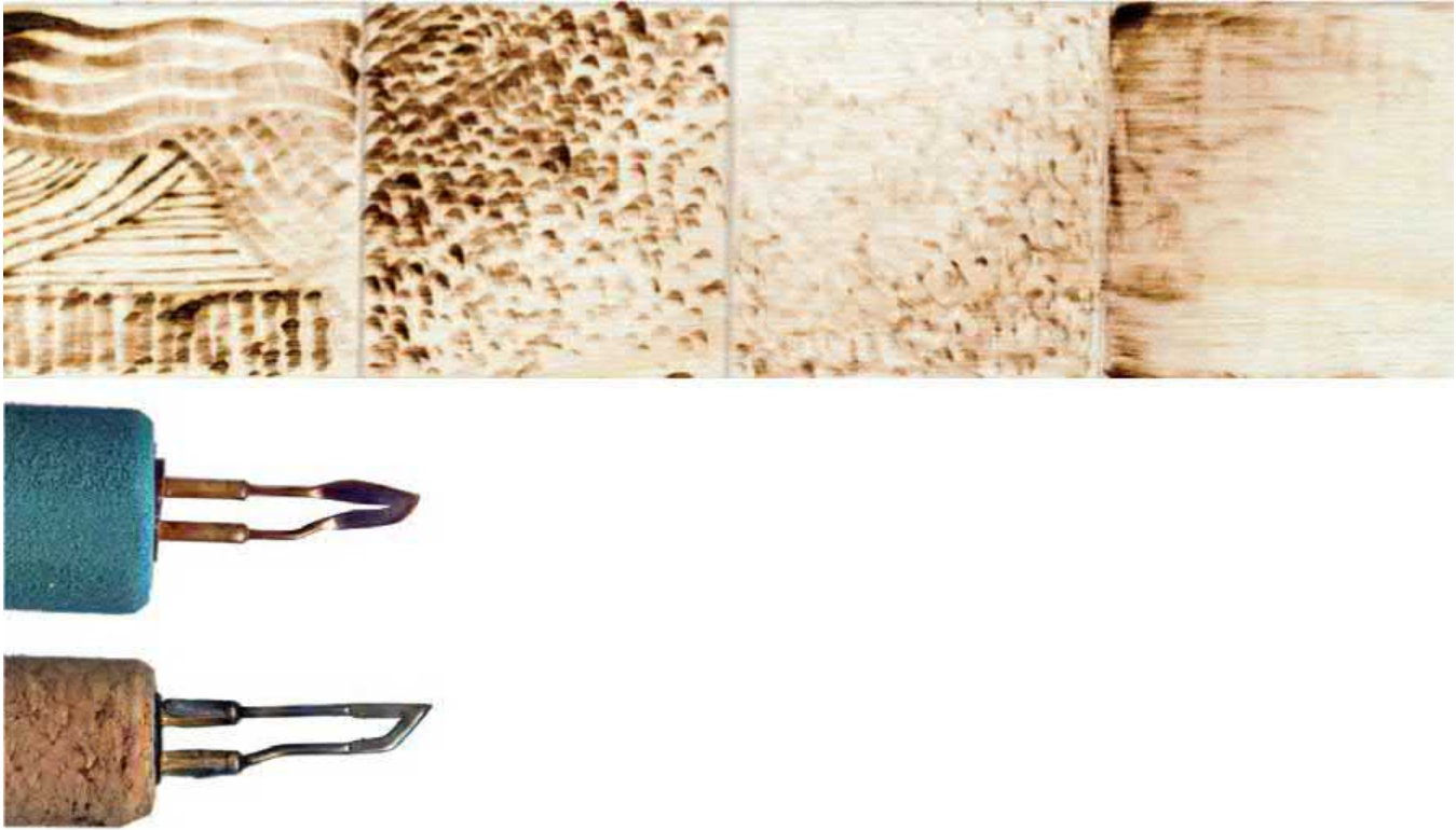
Figure 2.6. The touch-and-lift dot pattern of pointillism with this tip burns small triangles, as seen in square B. For D, the side of the spear shader is pulled so that the wide edge of the shader touches the board, creating a graduated, unlined shading effect.
