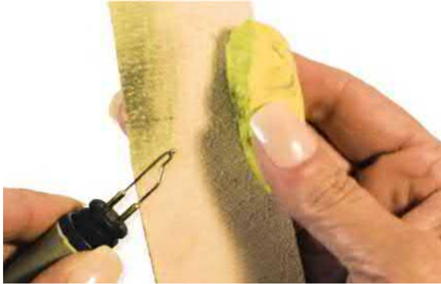
Figure 1.11. Yellow oxide rouging compound has been added to the raw side of this leather scrap. This will help remove the carbon build-up on wire-tip pens.
