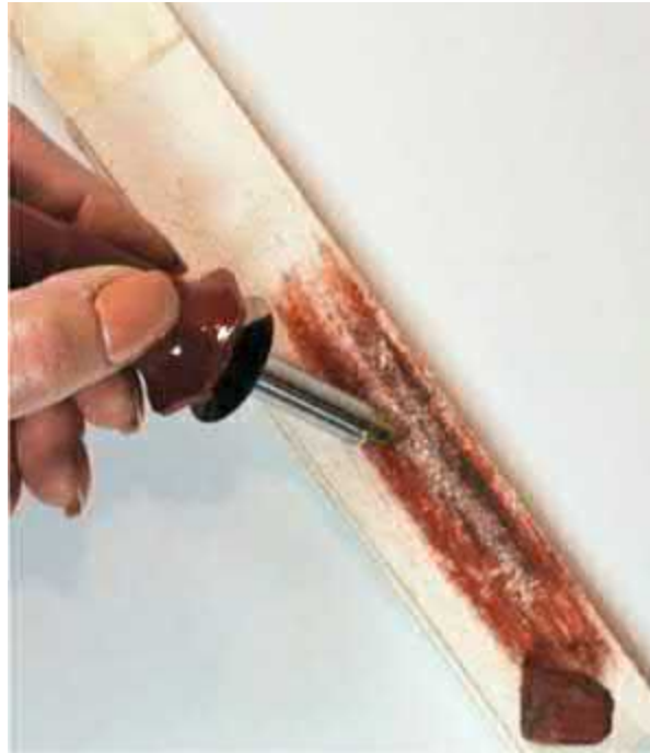
Figure 2.2. One-temperature and rheostat burning pens have a much thicker handle because that handle houses the burning unit. Although your fingers are wider apart than when using a variable-temperature pen, you use the same four-point grip.
