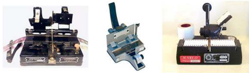
The Griswold, Cattozzo and Rivas 35 mm film splicers, each one named after the person who invented it
