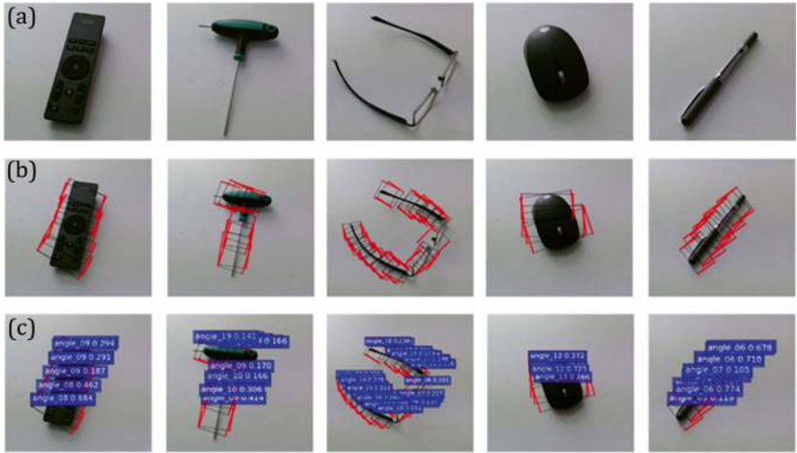
Fig. 5.20 Grasping frame prediction results under single item. (a) Original image of the item taken by Kinect V2; (b) Grasping prediction rectangle without marked score; (c) Grasping prediction rectangle with marked score
