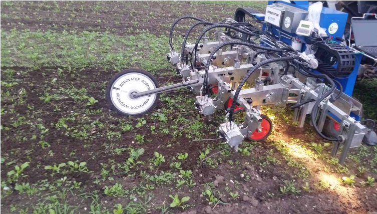
Figure 14 Robovator operating in weedy sugar beets. Courtesy of Frank Poulsen Engineering.
