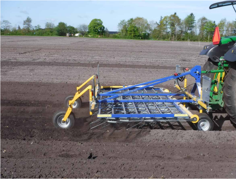
Figure 2 Weed harrowing on potato ridges with a Treffler harrow. Courtesy of Bo Melander, Aarhus University, Denmark.
