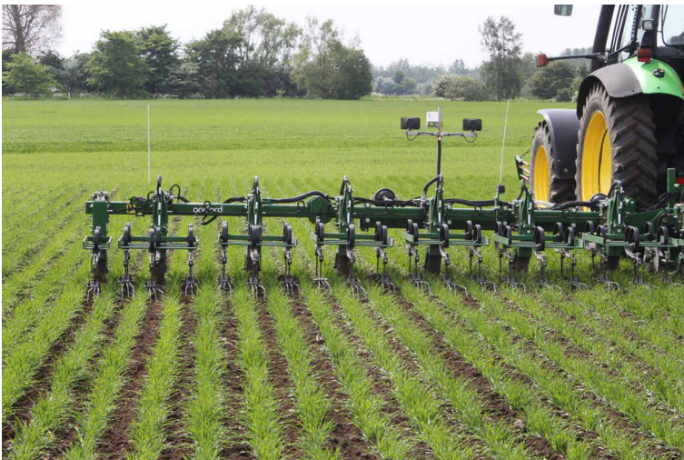
Figure 5 Camera-steered inter-row hoeing in spring barley. Courtesy of Bo Melander, Aarhus University, Denmark.
