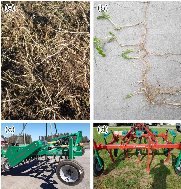
Figure 3 Reaching propagules below ground, (a) rhizomes of Elymus repens (photo Jukka Salonen), (b) adventitious roots of Cirsium arvense (photo Marian Weigel), (c) shallow cutting equipment (photo Jukka Salonen), (d) deep cutting equipment (photo Marian Weigel).
