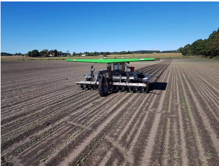
Figure 12 Farmdroid working in newly established winter oilseed rape. The oilseed rape was sown by Farmdroid and is now being inter-row cultivated – another possible application with the machine. Courtesy of Sven Hermansen, SEGES, Denmark.
