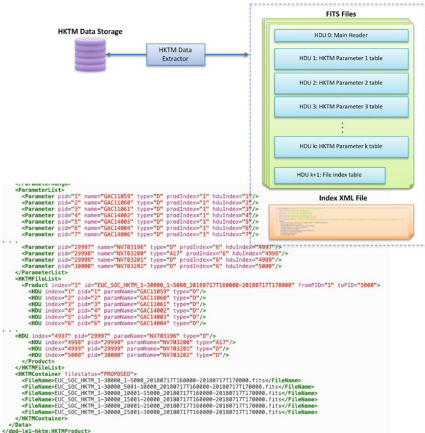
Fig. 11 HKTM product generation. Full HKTM is provided to the SGS as a FITS product, aggregating all HKTM cut per hour period. This allows later use decoupled from any Telemetry provision service
