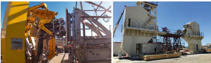
Fig. 8 ECT Fos-sur-Mer test set-up (ULPM on the left, LLPM on the right)
