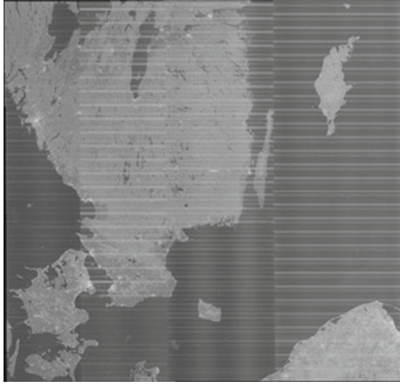
Fig. 4 Mutual radar interference between Sentinel-1a as seen from RADARSAT-2
