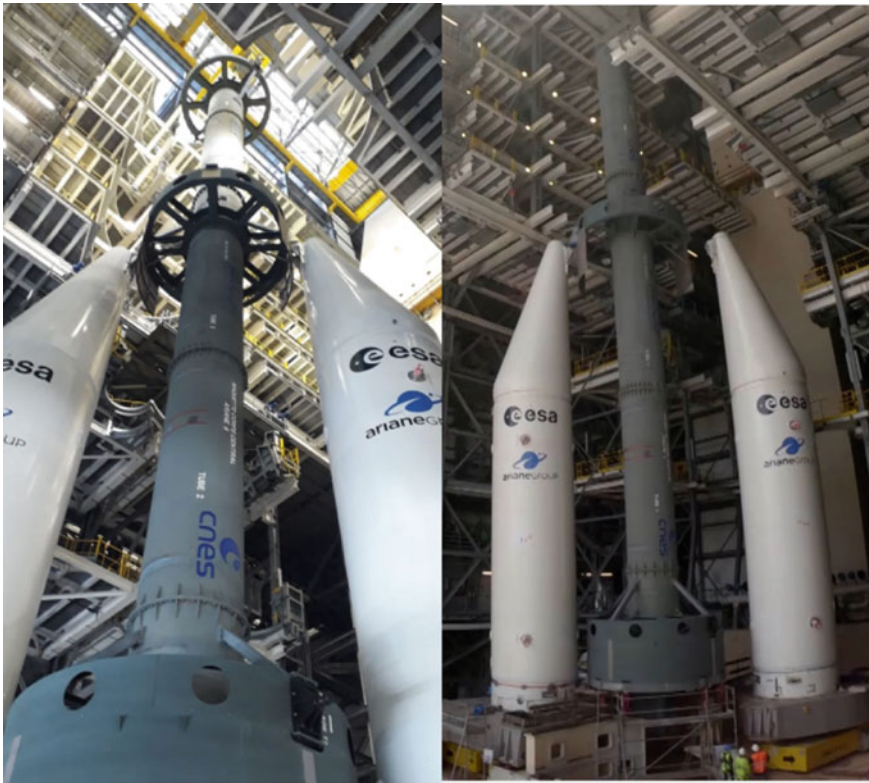
Fig. 10 ECT ESR/Central Core integration test set-up ©ESA/CNES/Arianespace
