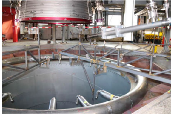
Fig. 6 ECT Vulcain 2.1 test set-up at DLR P5 test bench ©ESA/CNES/Arianespace
