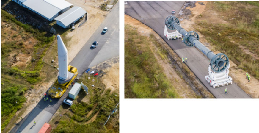
Fig. 14 Transfer test for LB transfer means technical qualification ©ESA/CNES/Arianespace
