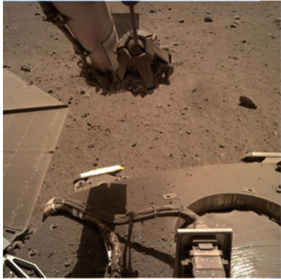
Fig. 29 After regolith deposit on the deck for solar array cleaning
