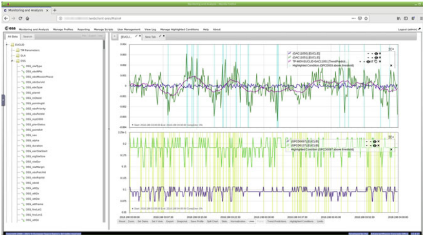
Fig. 7 WebMUST main screen showing the evolution of several parameters (Gaia mission data used for HKTМ) and grouping of parameters showing other source parameters as Survey (OSS) on the left pane
