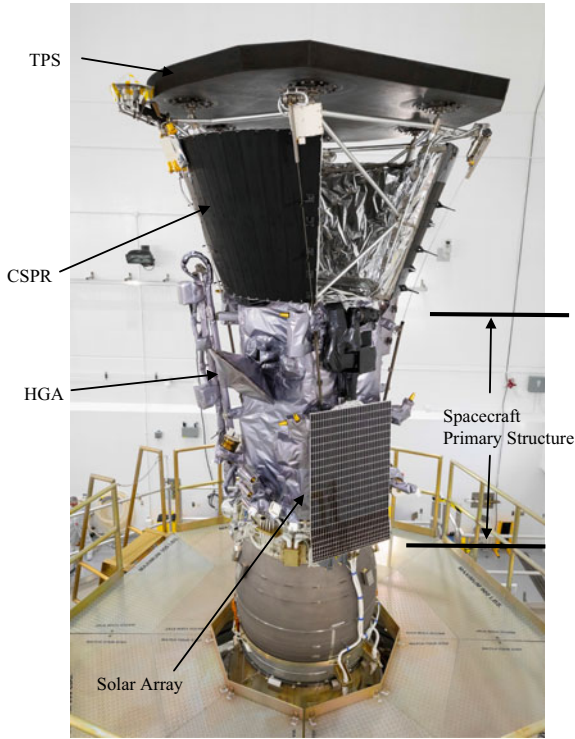
Fig. 3 PSP Installed on the 3rd Stage
