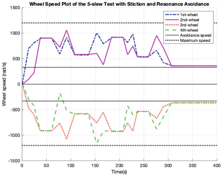
Fig. 8 Wheel speed plot for five consecutive slews using the stiction and resonance avoidance algorithm
