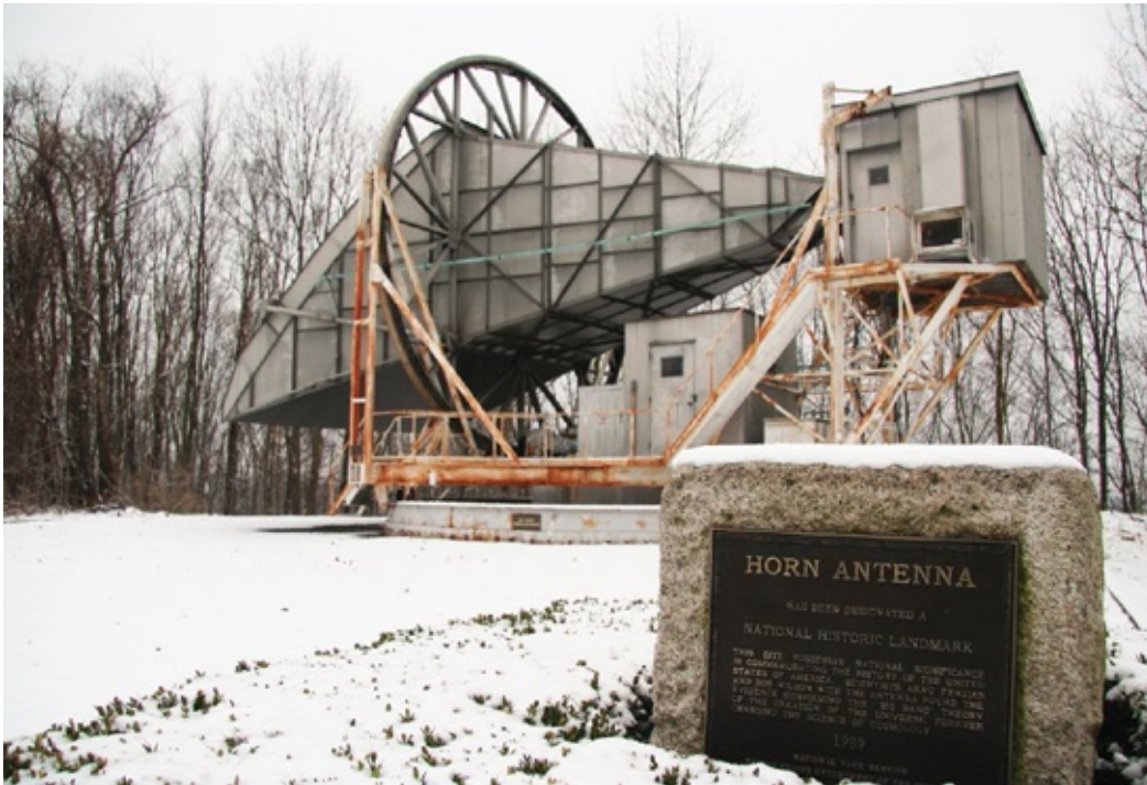
A photo of the historic horn-shaped radio antenna at Bell Labs in Holmdel, New Jersey, that was used by Arno Penzias and Robert Wilson to discover the faint glow of the cosmic microwave background emission that had been predicted by the big bang model for the origin of the universe.
