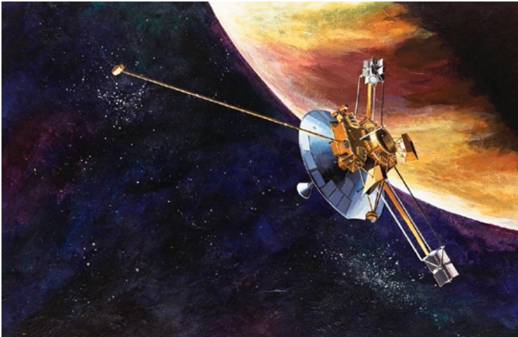
Artist's rendering of the Pioneer 10 spacecraft. The truss pointing down in this view is about 10 feet (3 meters) long.
