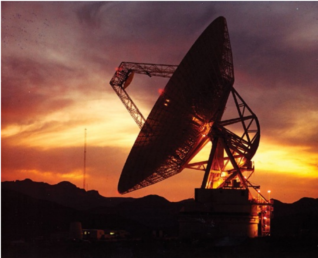
The 230-foot (70-meter) diameter radio telescope of the NASA/JPL Deep Space Network (DSN) at Goldstone, California. Similar DSN telescopes are located in Spain and Australia to maintain a constant vigil over humanity's fleet of interplanetary exploration spacecraft.
