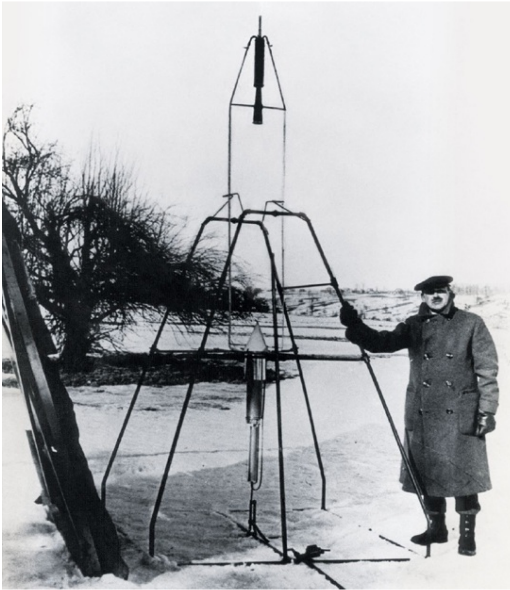
Robert Goddard poses with his first liquid-fueled rocket, which was launched from Auburn, Massachusetts, on March 16, 1926. Unlike conventional rockets today, this model's combustion chamber and nozzle were at the top, and the fuel tank below. It flew for 2.5 seconds and rose 41 feet (12.5 meters).
