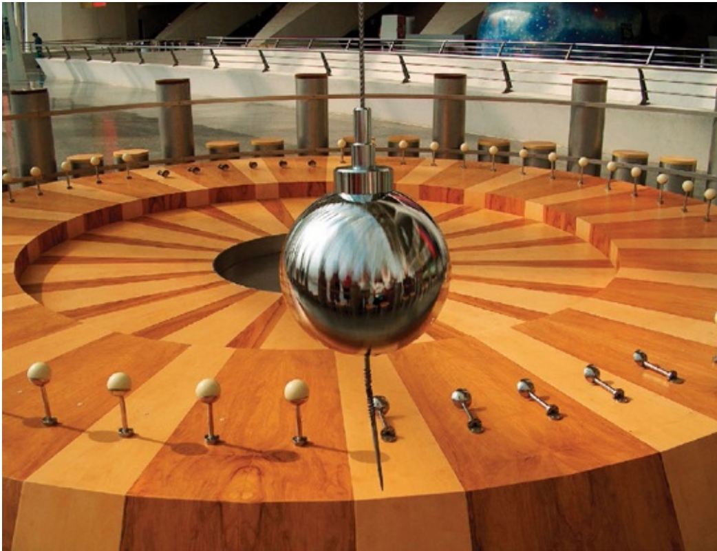
A large Foucault pendulum from the Príncipe Felipe Science Museum of the City of Arts and Sciences in Valencia, Spain. In this setup, a little ball and stick model is tipped over roughly every 30 minutes because the Earth is spinning underneath the inertially fixed plane of the pendulum's swing.
