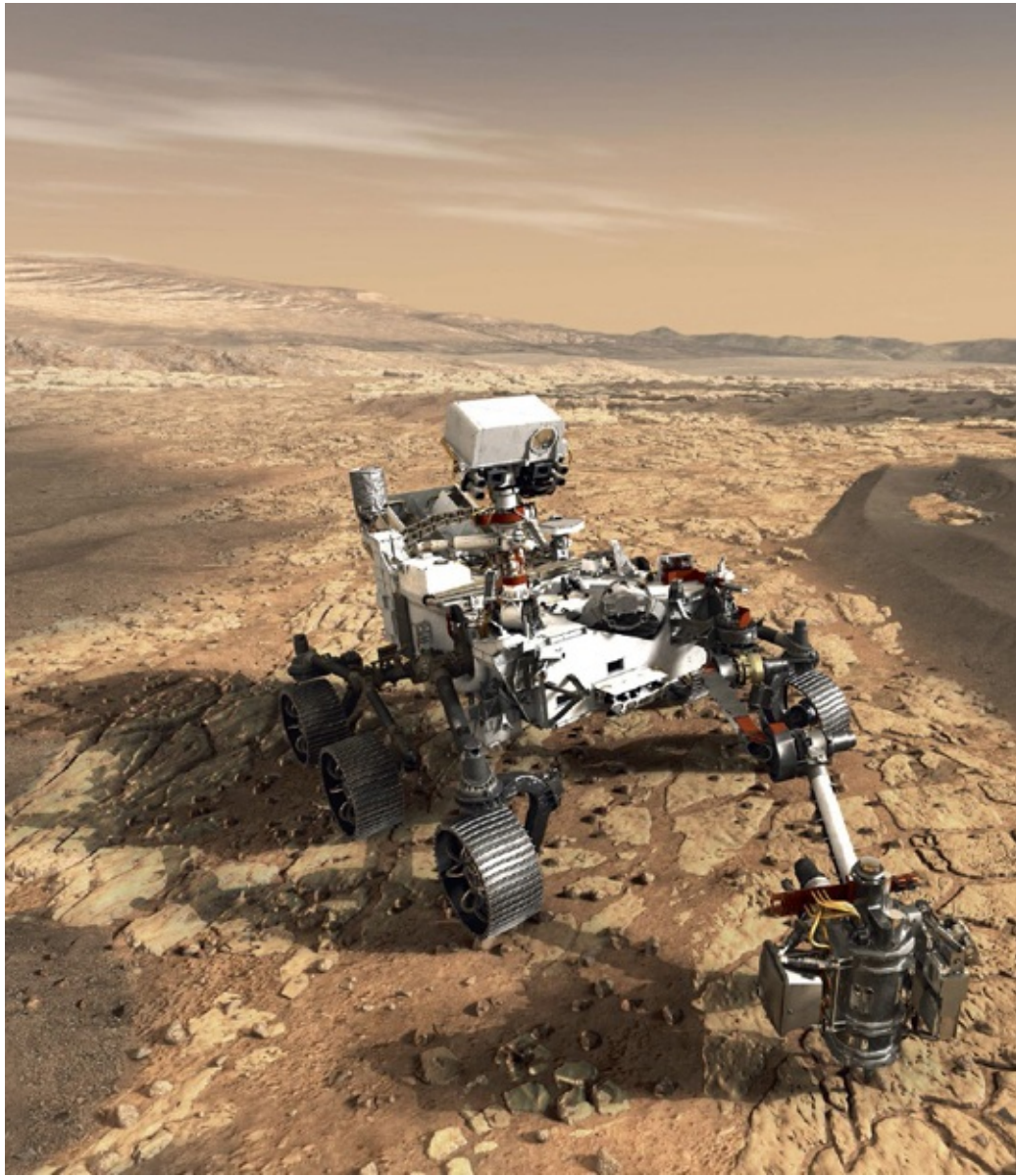
Artist's rendering of the NASA Mars 2020 rover, drilling a rock core to be cached for a later mission to return to Earth.
