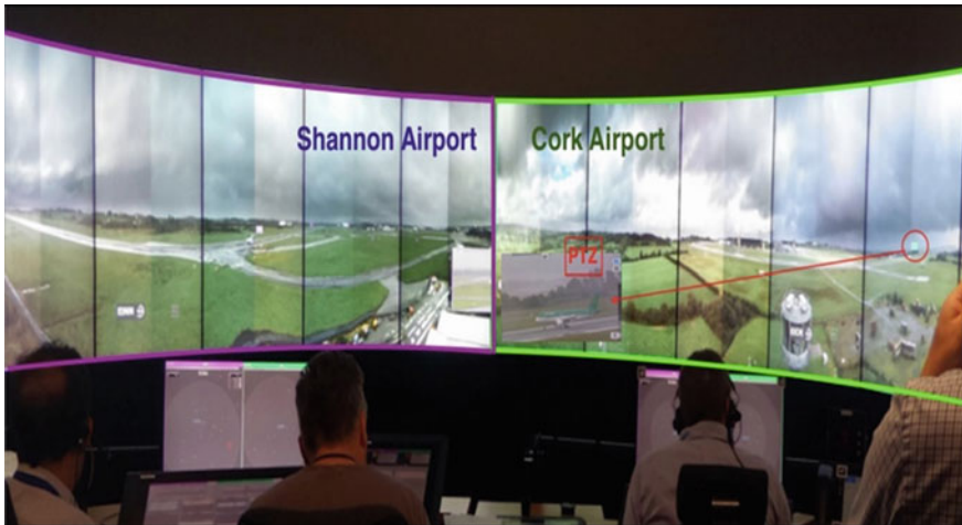
Fig. 1 The multiple remote tower operational centre equipped with PTZ, EFS, RDP and OTW located at Dublin Airport provided air traffic services for both Shannon and Cork airports simultaneously by SAAB digital tower systems
