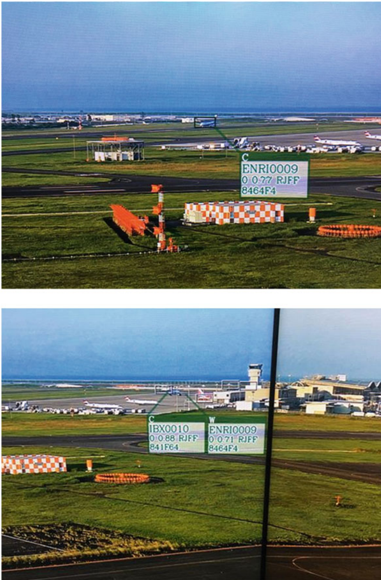
Fig. 12 Examples of object detected by image processing labelled with MLAT information
