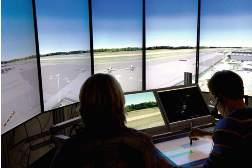
Fig. 14 RTC-HFS: remote tower controller working position (CWP-) design
