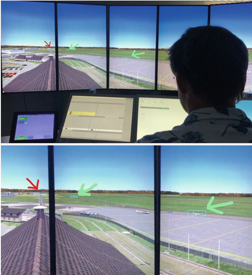
Fig. 1 Experimental set up of the Remote Tower Module with Tracking Boxes in the Panorama Visual Presentation remark: two tracking boxes on the taxiway are “wanted” [green arrows], the one in the back is an unwanted “nuisance” tracking box [red arrow]; the figure below shows a magnification of the scenery above
