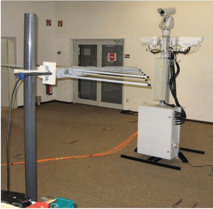
Fig. 12 Experimental setup for measuring electromagnetic emission
