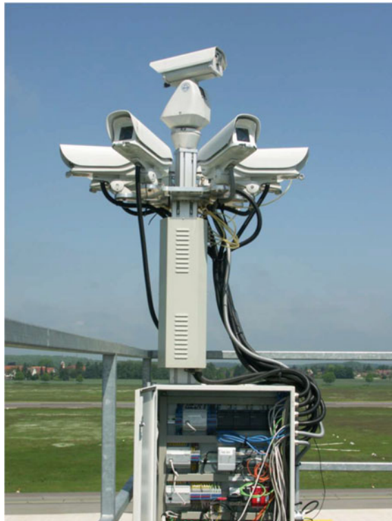
Fig. 2 Panorama camera and PTZ setup at the Airport Braunschweig/Wolfsburg
