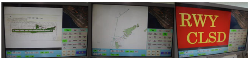
Fig. 9 Examples of the MPID display can show AIP such as airport map and charts and status check list of operation
