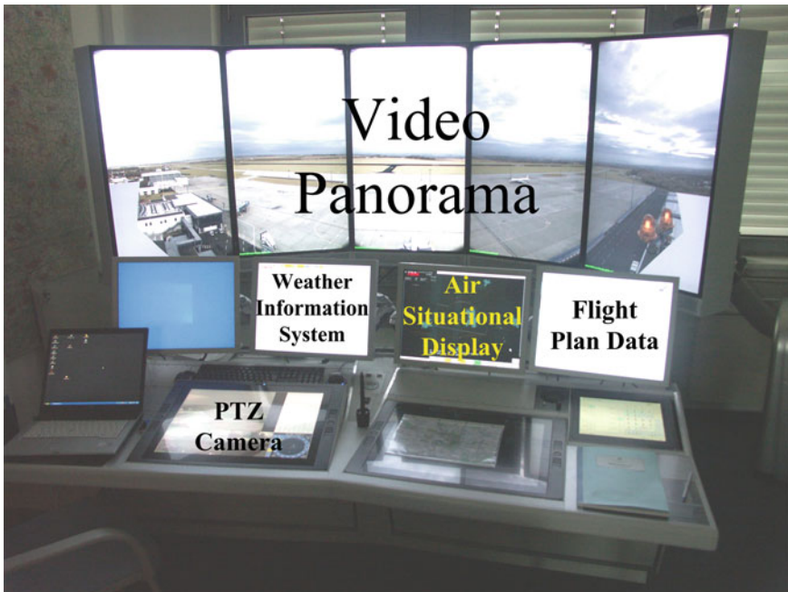
Fig. 2 CWP-remote at the airport Erfurt
