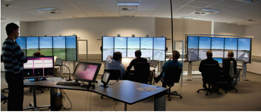
Fig. 15 Remote tower center (RTC) design for controlling three airports from afar. Foreground: ground coordinator; back: three airport CWP's for executive controllers
