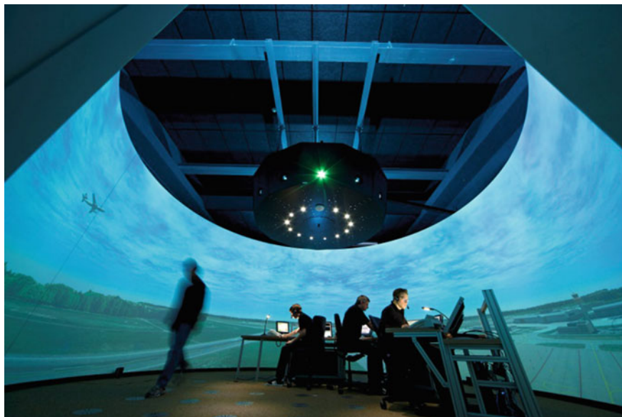
Fig. 10 ATS360: the close-to-reality apron and tower simulator of DLR
