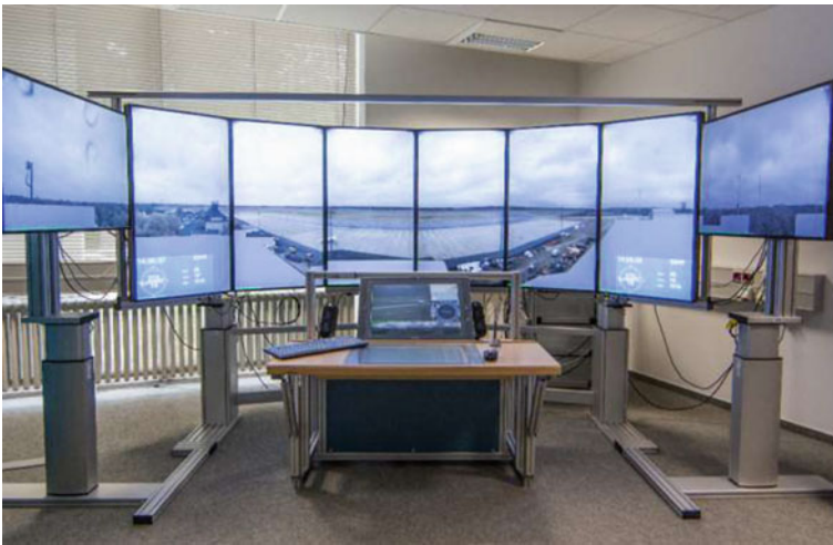
Fig. 3 Prototype RTO-Video panorama with basic controller console in the DLR Tower-Lab (2013) reproducing the out-of-windows view at Braunschweig airport. 360° horizontal FOV with 6 vertical displays for the 228° view towards the runway in northern direction. Two horizontal displays covering the southern 136° viewing sector with the same resolution
