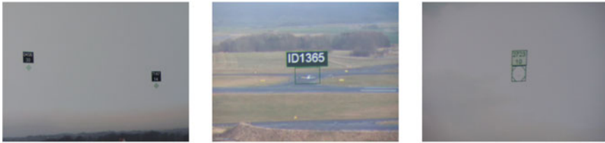
Fig. 5 Left: Aircraft tracked only by the Terminal Approach Radar (labels with call sign or SSR code and altitude in hundreds of feet); Middle: aircraft tracked by the video camera only (label with track number); Right: aircraft tracked by both radar and video
