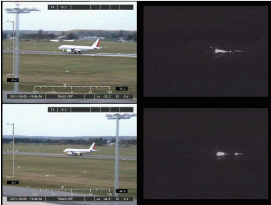
Fig. 11 Thermal Image of turbine exhaust without (upper images) and with reverse thrust activated (lower images)
