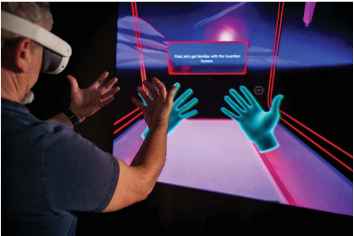
FIGURE 5.4 Gesture recognition by HMD cameras. (Credit: Krzysztof Pagacz.)
