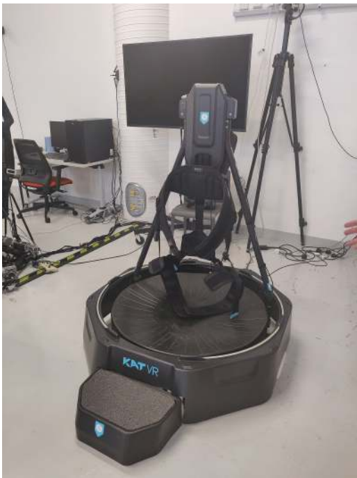
FIGURE 6.1 KAT Walk omnidirectional treadmill supporting hardware-assisted locomotion in virtual reality. (Photo: Tim Sheerman-Chase, CC BY 2.0, Wikimedia Commons [ https://commons.wikimedia.org/wiki/File:Treadmill_Omni.jpg ].)
