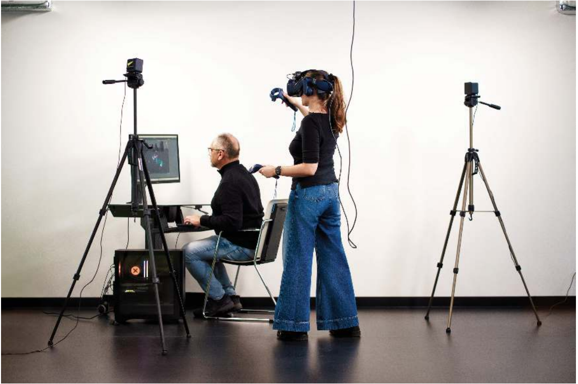
FIGURE 0.10 HTC Vive headset and Lighthouse tracking system enabling room-scale VR.
