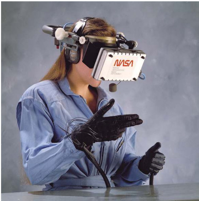
FIGURE 0.5 The VIEW (virtual interactive environment workstation) system developed at NASA Ames Research Center in the late 1980s. The operator uses a head-mounted display together with DataGlove controllers to interact with a virtual environment. (Source: Wikimedia Commons [ https://commons.wikimedia.org/wiki/File:THE_VIEW_(Virtual_Reality).jpg ].)
