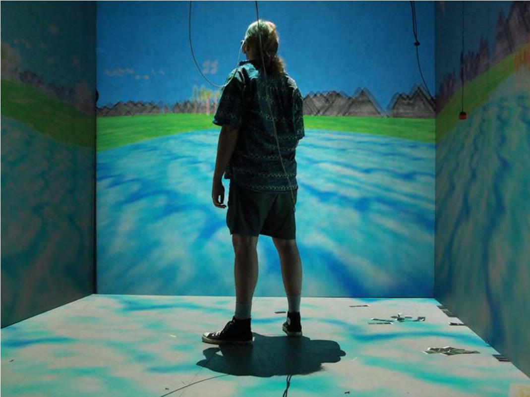
FIGURE 0.6 CAVE (cave automatic virtual environment), an immersive projection-based virtual reality system in which stereoscopic images are displayed on the walls of a room-sized cube, allowing users inside the environment to explore virtual scenes without wearing a head-mounted display. (Source: Wikimedia Commons [ https://commons.wikimedia.org/wiki/File:CAVE_Crayoland.jpg ].)
