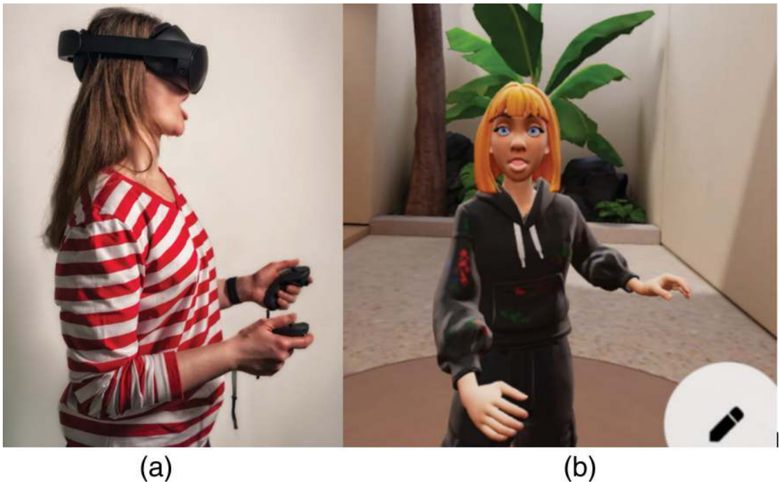
FIGURE 15.8 Example of facial expression tracking and real-time avatar animation in Meta Quest Pro.
