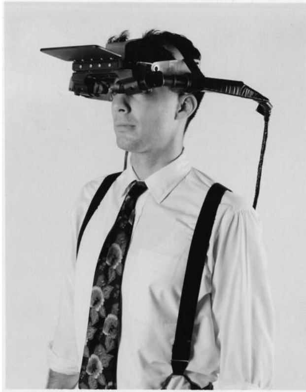
FIGURE 0.4 The “Sword of Damocles” head-mounted display developed by Ivan Sutherland in 1968, considered the first computer-based virtual reality system capable of displaying computer-generated graphics aligned with the user’s head movements. (Image courtesy of the Computer History Museum, https://www.computerhistory.org/revolution/input-output/14/356/1888 )
