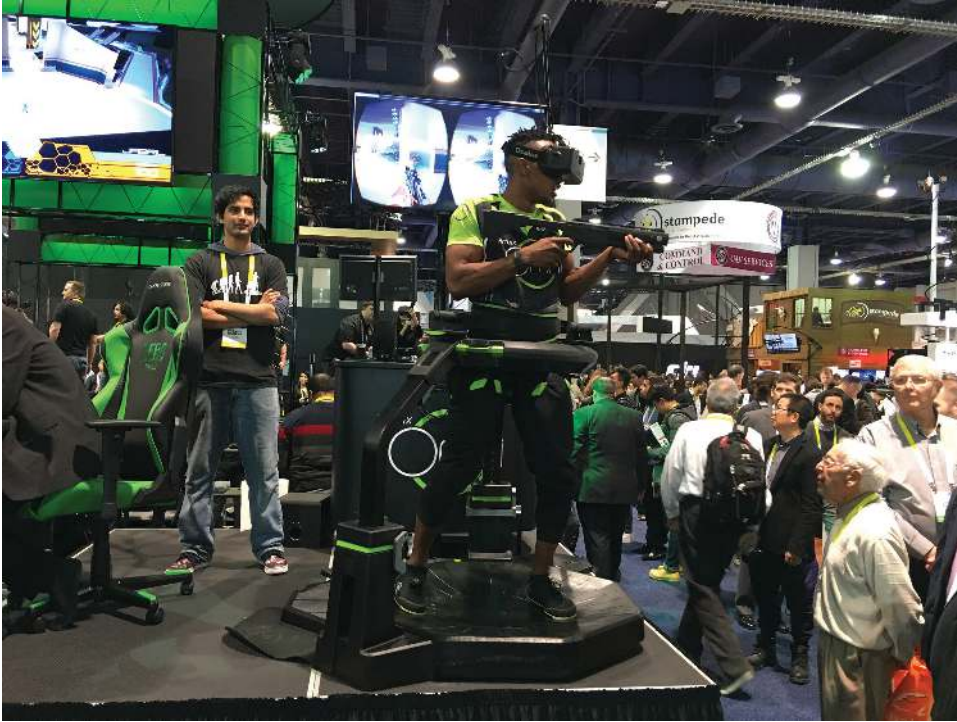
FIGURE 6.2 Virtuix Omni omnidirectional treadmill in use during public demonstration. (Photo: tomemrich, CC BY 2.0, Wikimedia Commons [ https://commons.wikimedia.org/wiki/File:Treadmill_Omni.jpg ].)
