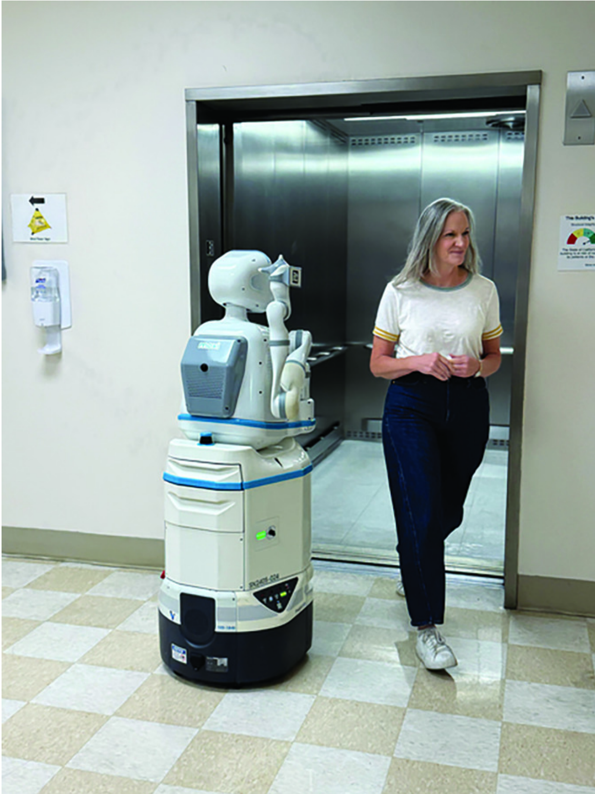
Figure 8.1 Moxi robotic assistant by Diligent Robotics can fetch items for staff and independently navigate in a hospital.
