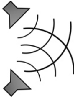
Figure 10.19: Two speakers out of phase; phases do not add constructively. ↗
