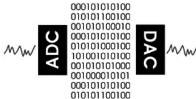
Figure 3.2: A pictorial description of the recording and playback of sounds through an ADC/DAC. ↗
