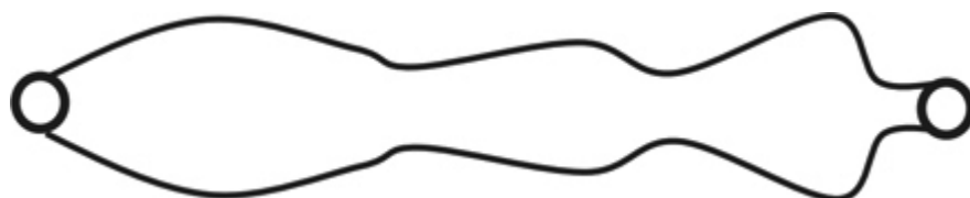
Figure 9.4: The physical analogy of LPC: a tube with varying cross-section. ↗
