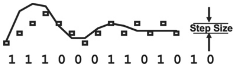
Figure 13.2: DPCM. The solid line is encoded into 1’s and 0’s shown below. The reconstructed signal is shown as small boxes. Each box is at the value of the previous one plus or minus the step size. ↗
