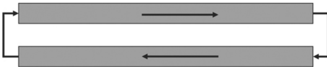
Figure 11.4: A waveguide model. The right-going and left-going wave, which are superimposed on a single string, are modeled separately as simple delays. The signal connections at the ends of the delays represent reflections. A waveguide can also model a column of air as in a flute. ↗
