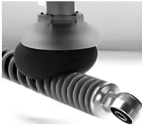
Figure 10.1(a): A spherical-type soft gripper (Zhao et al., 2021). ↗
