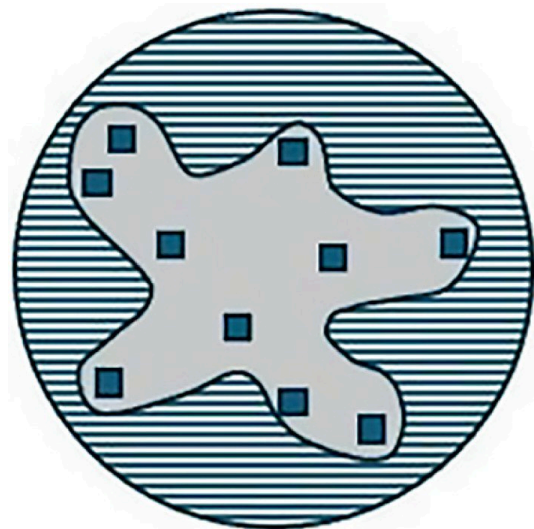
Fig. 1.11 Overfitting: Small squares represent correct instances given to the system. If the system tries to be precise only for those instances, the result of learning is too narrowly focused on the target area
