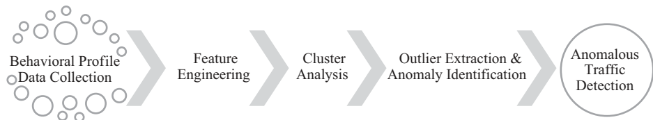
FIGURE 7.6 Process for detecting anomalous traffic using clustering algorithms.
