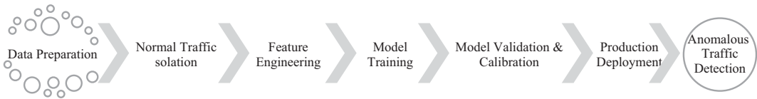
FIGURE 7.10 Overall process for anomalous traffic detection using the One-Class SVM algorithm.
