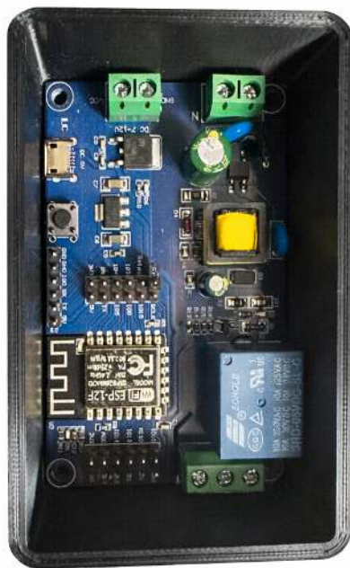
Figure 5.12 – Box with lid being printed and electronic board fitment check
