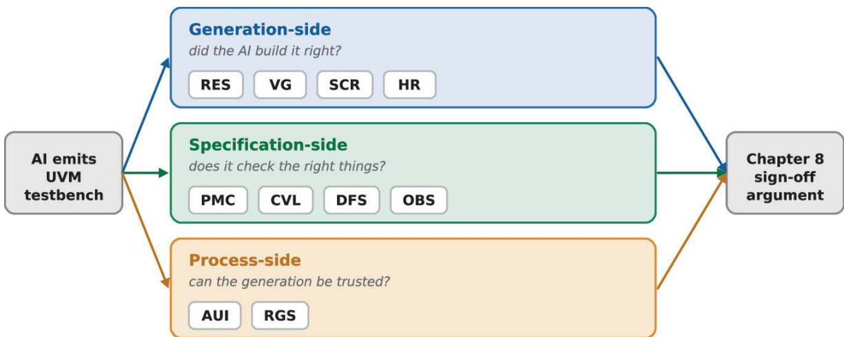
Fig. 7.1 The three metric families and the question each answers. After the AI emits the testbench, the generation-side family (RES, VG, SCR, HR) grades whether it runs, the specification-side family (PMC, CVL, DFS, OBS) grades whether it checks and can observe the right things, and the process-side family (AUI, RGS) grades how much of the output was trusted and how repeatable it is. All three feed the sign-off argument of Chap. 8
