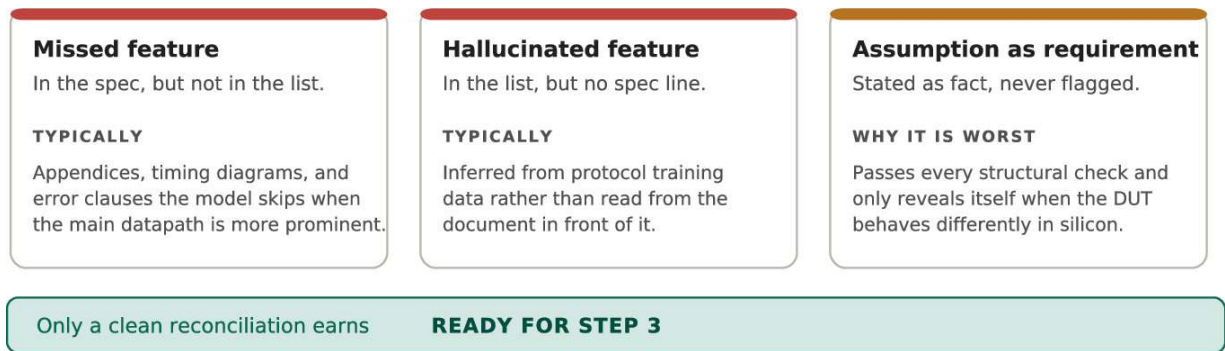
Fig. 2.2 Reviewing the feature list against the spec. Three failure classes hide in the gap: features in the spec but missing from the list, features in the list with no spec line, and assumptions stated as requirements. Only a clean reconciliation earns READY FOR STEP 3
