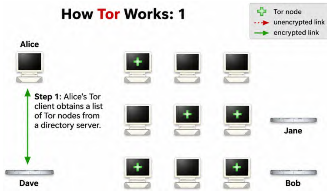
Figure 12.13: Step 1 of how Tor works: Alice's Tor client obtains a list of Tor nodes from a directory server.
