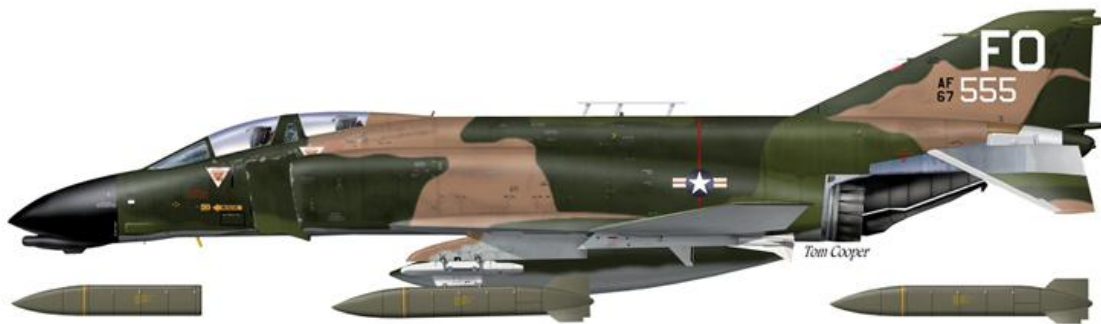
F-4D FO, 66-7555, 435th TFS/8th TFW – this is one of the few LORAN-equipped examples (shown with two variants of the SUU-13 dispenser pod family). The bigger pod is the SUU-41 – and the example is shown installed on a TER The SUU-41 was the so-called ‘Gravel Pod’ about which little is known. In essence, these dispensers were literal ‘flying refrigerators’ and were filled with liquid Freon in which various experimental weapons were then ‘dipped’, such as the XM40E5 Sandwich button bombs; XM44 electronic anti-intrusion devices; and even the XM48 mechanical button bomblets (gravel mines). In the lower-left corner we see a similarly-shaped, but smaller, SUU-33 CBU which was filled with anti-vehicle mines.
