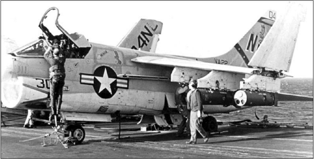
An A-7E from the VA-22 of the USS Coral Sea is seen being loaded with Mk-55 aerial mines following President Nixon's orders to mine the Haiphong Port, as well as the less important harbors of North Vietnam. (US Navy)
