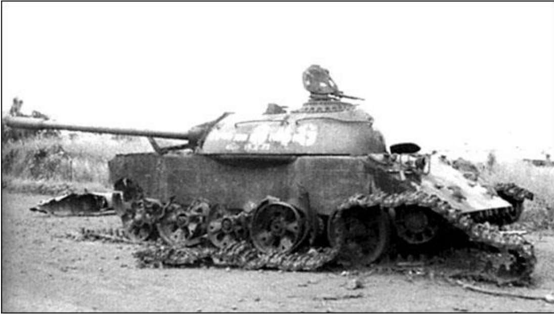
Another T-54B belonging to the 20th Tank Battalion destroyed on the outskirts of An Loc. It was hit by an anti-tank rocket that ignited its internal ammunitions. (US Army)
