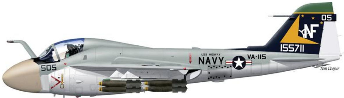
USN A-6A, NF505; VA-115 'Arabs' was deployed as part of air wing CVW-5 on board USS Midway (CVA-41) off Vietnam from April 1972 until March 1973. The plane is shown carrying a MER with six Mk-82 GP bombs equipped with Mk.15 Snakeye retarding fins.
