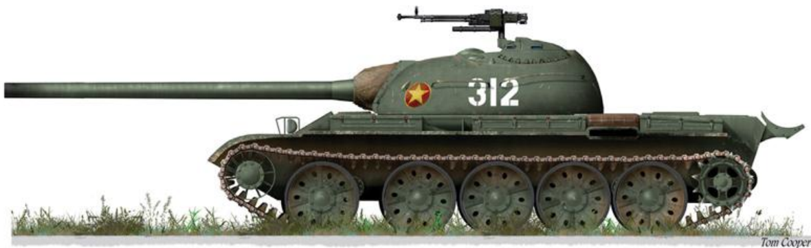
T-54A number 312 of the PAVN 21st Armored Battalion, An Loc – June 1972. This machine formed part of one of the first batches of T-54s delivered to North Vietnam in 1964 and was still in service. Note that there are no ‘smoke-evacuators’ on the gun barrel, and the old wheels.
