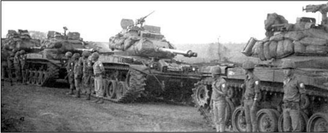
The M41A3s of a tank troop belonging to the 19th ACS move out of Kontum to be redeployed to Tan Canh near the ARVN 22nd Division advanced Command Post. Note the sandbags installed around the turrets for additional protection against the RPG shaped-charge rockets. (US Army)
