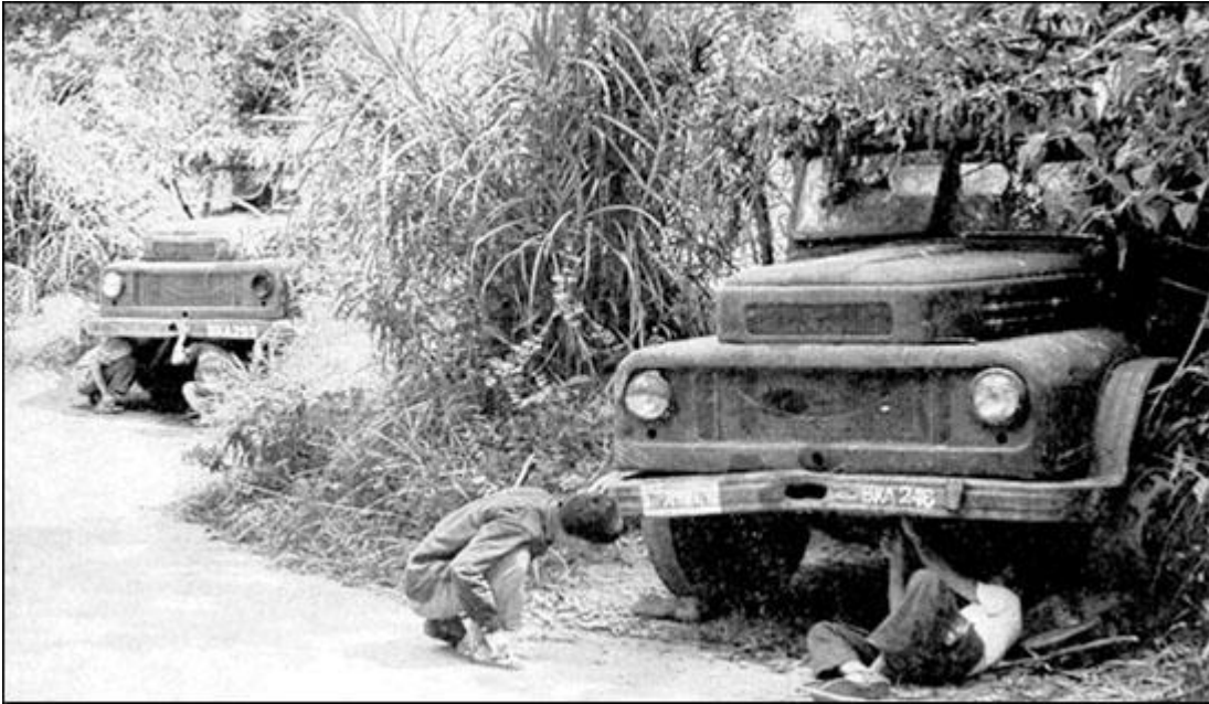
Drivers of the PAVN 2nd Division check the status of their North Korean-built Sunghri 58KA trucks of 2.5-ton capacity. Pyongyang delivered more than 2,000 of them to Hanoi for the 1972 campaign. (PAVN)
