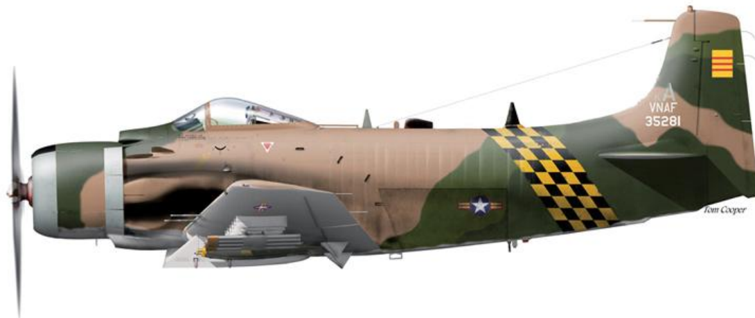
VNAF A-1H, serial 135281, of the 514th Fighter Squadron from the 23rd Tactical Wing of Bien Hoa AB – May 1972. It was armed with Mk-82 HE bombs and CBU-25 dispensers.
