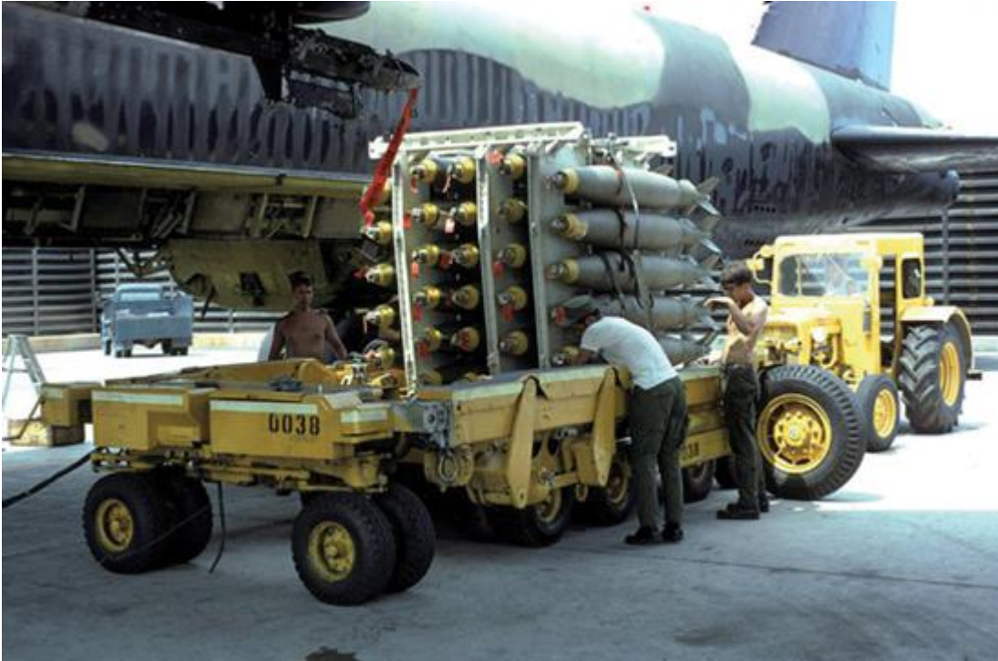
These armourers are loading a B-52D bomber. The aircraft typically carried a load consisting of no less than 108 bombs, including eighty-four 500lb and forty-two 750lb munitions. Their round the clock bombardments broke the back of the North Vietnamese divisions. (USAF)
