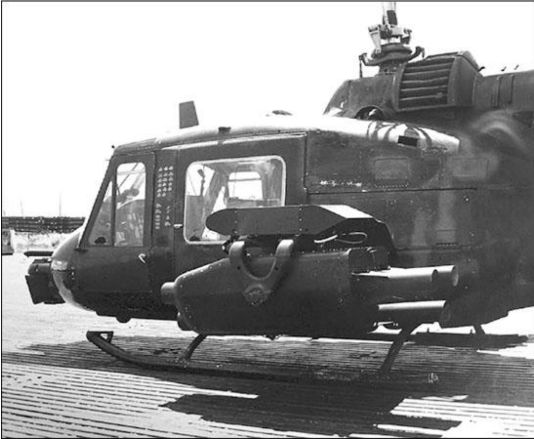
One of the two NUH-1B helicopters from the 1st Combat Aerial TOW Team which is deployed to Kontum to test the new wire-guided anti-tank missile. The unit claimed a total of 47 kills, including 24 tanks. (US Army)
