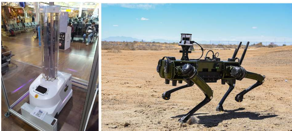
FIGURE 5.2: Robots use probability distributions to recognize objects and navigate surroundings. Left: Heathrow Airport has eight ultraviolet-disinfecting (UVD) robots that roam the terminals to clean and disinfect (Mx. Granger, Wikimedia Commons). Right: A Vision 60 Q-UGV ground robot does a simulated route mission at Holloman Air Force Base, New Mexico, April 17, 2023 (U.S. Air Force photo by Airman 1st Class Isaiah Pedrazzini, Wikimedia Commons). 📄
