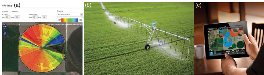
FIGURE 3.5 (a) Variable prescription over a storage capacity map; (b) center-pivot with section-by-section variable irrigation; (c) irrigation control on a web platform. (From TristateKS; Lindsay.)
