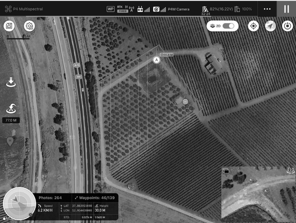
FIGURE 5.8 DJI flight-planning software interface.
