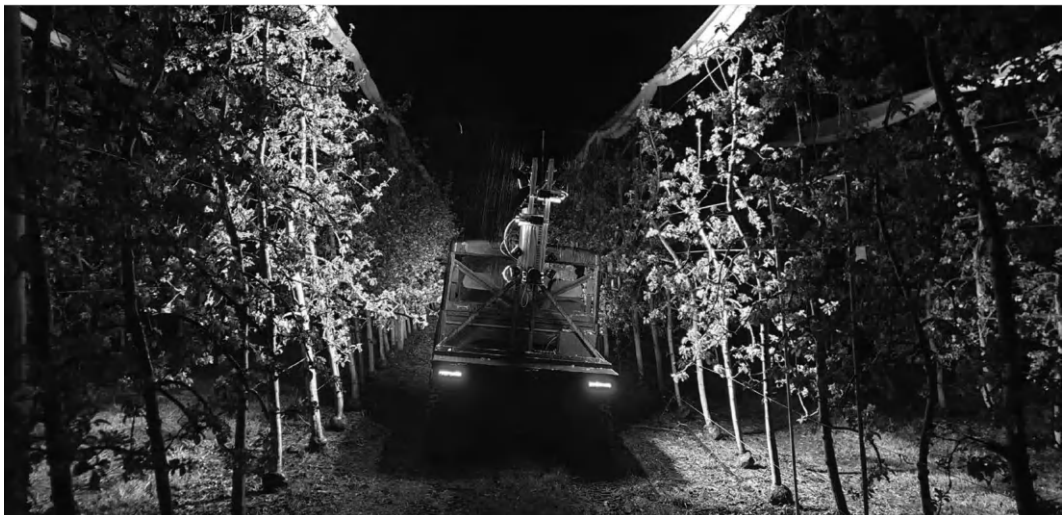
FIGURE 2.4 Ruggedized data capture rig with machine vision cameras working at night.
