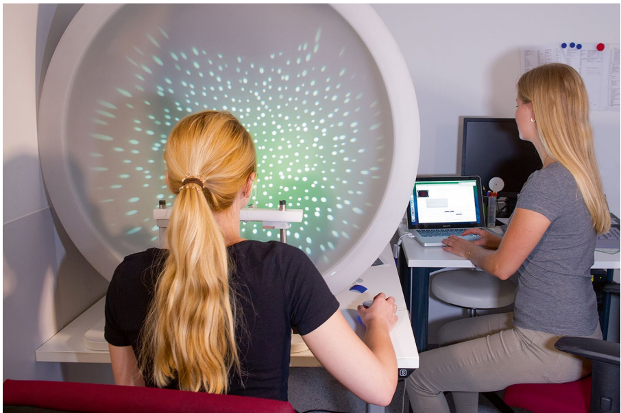
Fig. 2.6 Instrumental measurement of the subjective visual vertical using a hemispheric dome and light dots to measure perceived verticality
