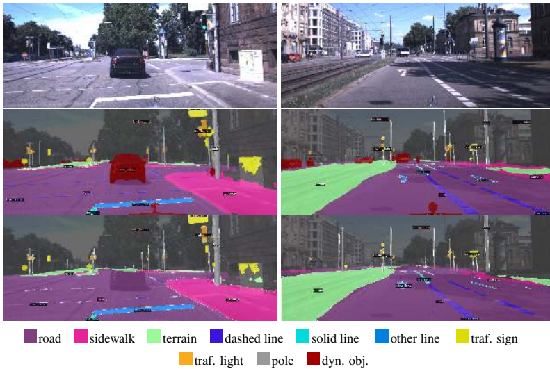
Figure A.5: Qualitative evaluation of dynamic occlusion handling. Two prediction examples are shown for a model trained with dynamic occlusion handling and without. Top to bottom: RGB image, prediction results of model trained with dynamic occlusion handling, prediction results of model trained without dynamic occlusion handling. Both examples are from the geo.-split test set.
