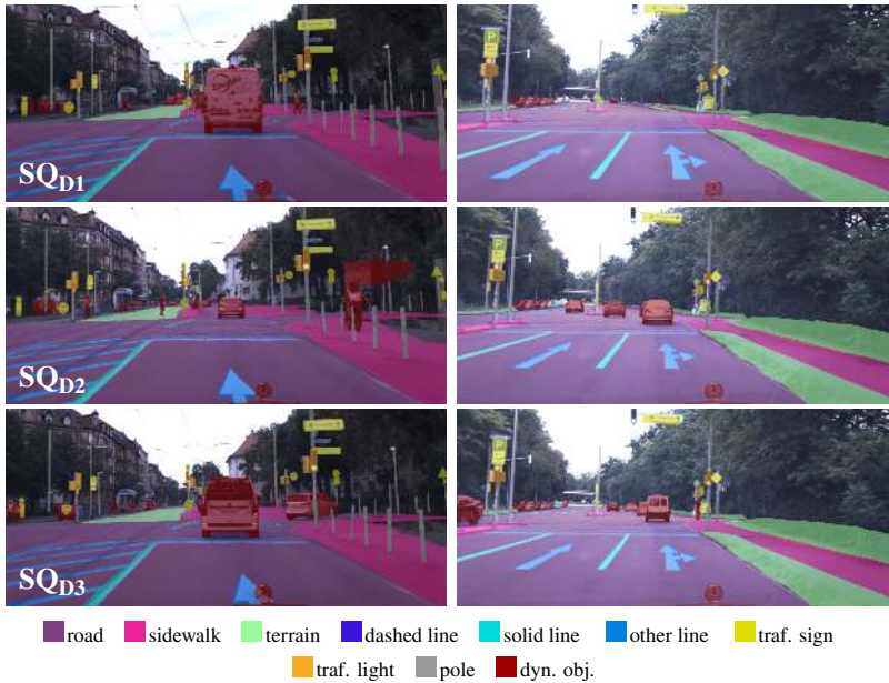
Figure 5.12: Qualitative evaluation of multi-drive mapping precision by assessing rendered map features in three drives of the same sequence. Left and right show two different scenarios and top to bottom depicts the same scenario in three different drives.
