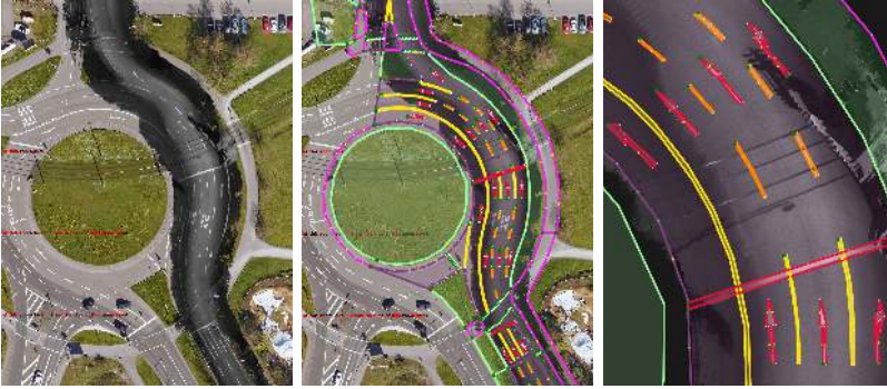
Figure 5.4: Annotation process of dense road surface features. Left: overlay of reconstructed road surface and aerial imagery, middle shows the annotated road surface features and right shows the same features in a zoomed-in view. The color coding is explained in Table A.3. Imagery: ©Stadt Karlsruhe | Liegenschaftsamt.
