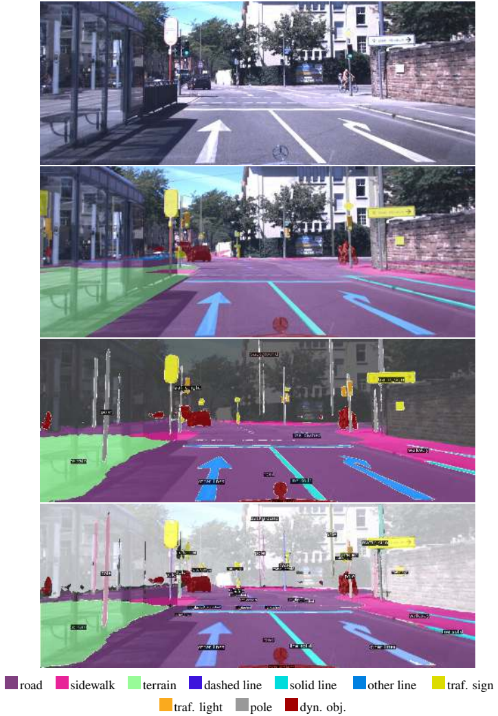
Figure 7.7: Qualitative evaluation of perspective panoptic segmentation. Top to bottom: RGB image, annotated ground truth, prediction results of panoptic segmentation shown as semantic masks and full panoptic output. Examples are from the geographically distinct test set.
