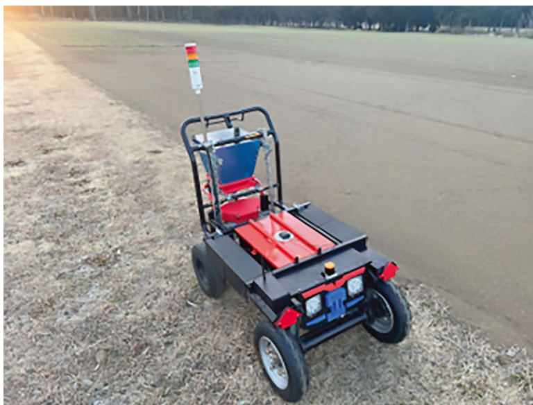
Fig. 16.7 Warning light tower implemented small-scale autonomous seed broadcasting vehicle (University of Tsukuba, Ibaraki, Japan)
