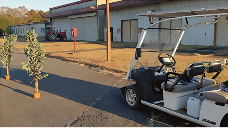
Fig. 9.15 Simulated environment for automated spraying testing using fake trees and a golf cart. The spray nozzles have been fixed to the rear of the cart
