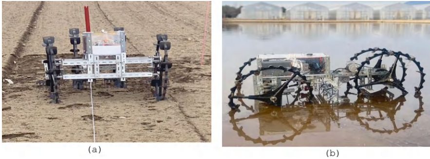
Fig. 17.8 (a) Assembly of the autonomous weeder for dryland fields and (b) assembly of the autonomous weeder for dryland fields
