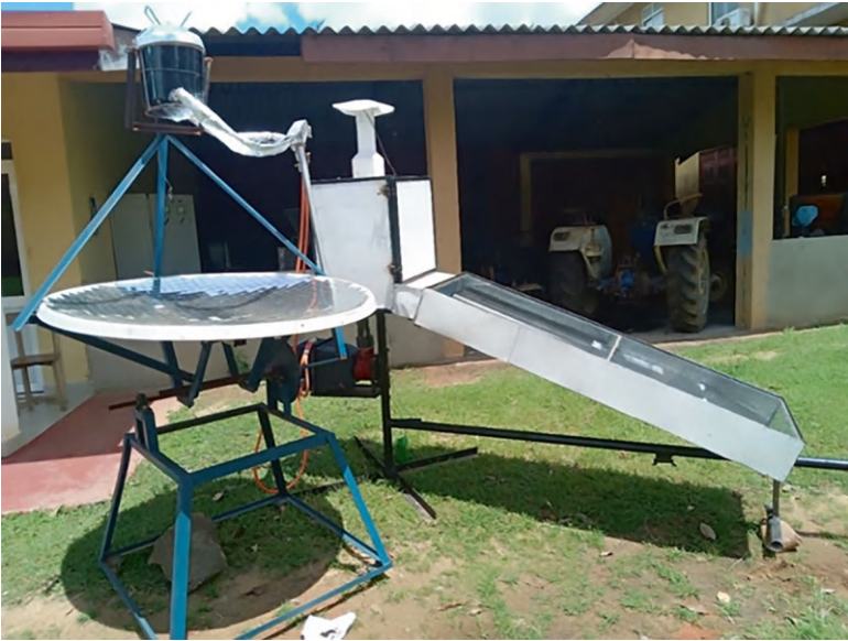
Fig. 20.10 Fabricated IoT-assisted dual solar supply dryer
