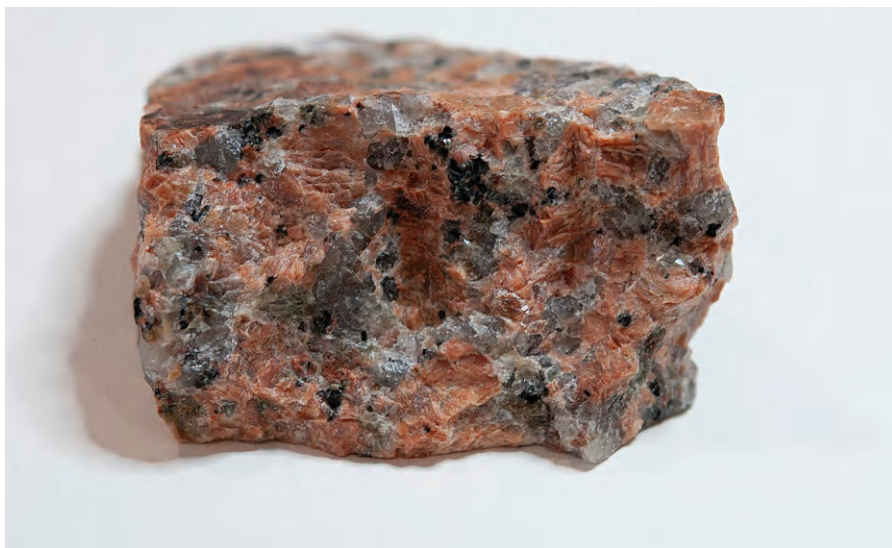
FIGURE 2.1 The interlocking crystals within a granite. The orange crystals are orthoclase, the clear greyish crystals quartz and the dark crystals biotite.
