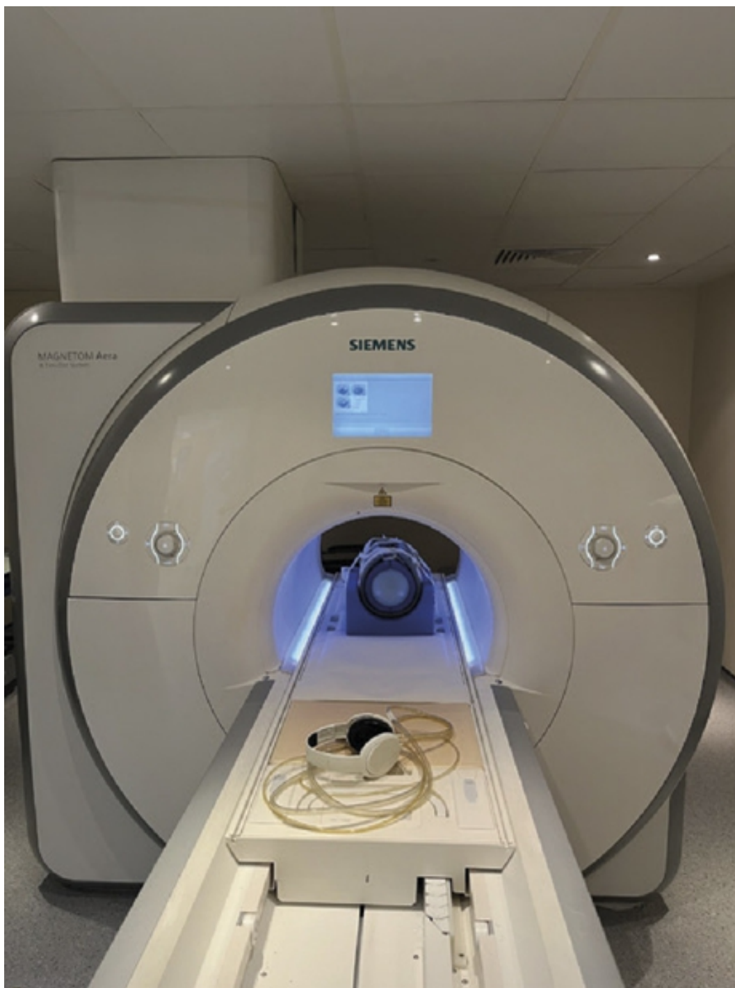
Fig. 1.6a Typical setup of a body array coil phantom QA test. 🔗
