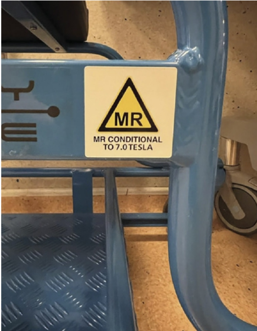
Fig. 1.9c MR Conditional label affixed to an MR-compatible trolley. ↗
