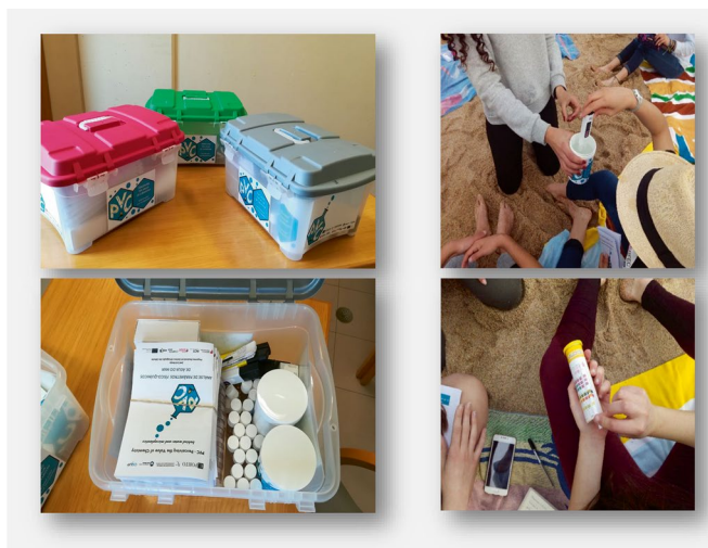
Fig. 6.5 PVC citizen science project: kits developed for the collection and analysis of certain physico-chemical water quality parameters
