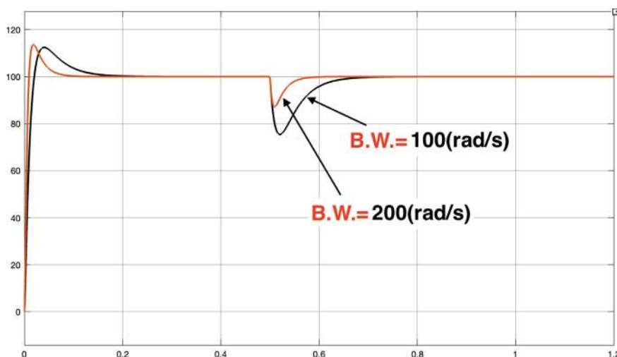
Fig. 2.56 Speed response waveforms using different PI controller gains
