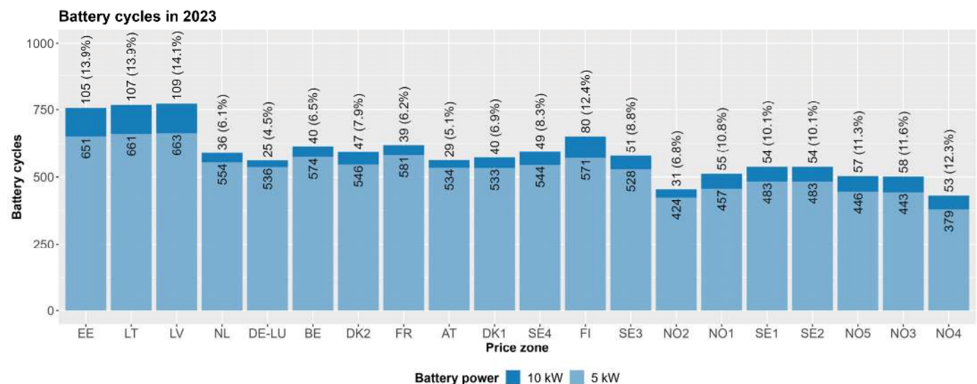
Figure 6. Total battery cycles increase by using a 10 kW power battery compared to a 5 kW power battery.
