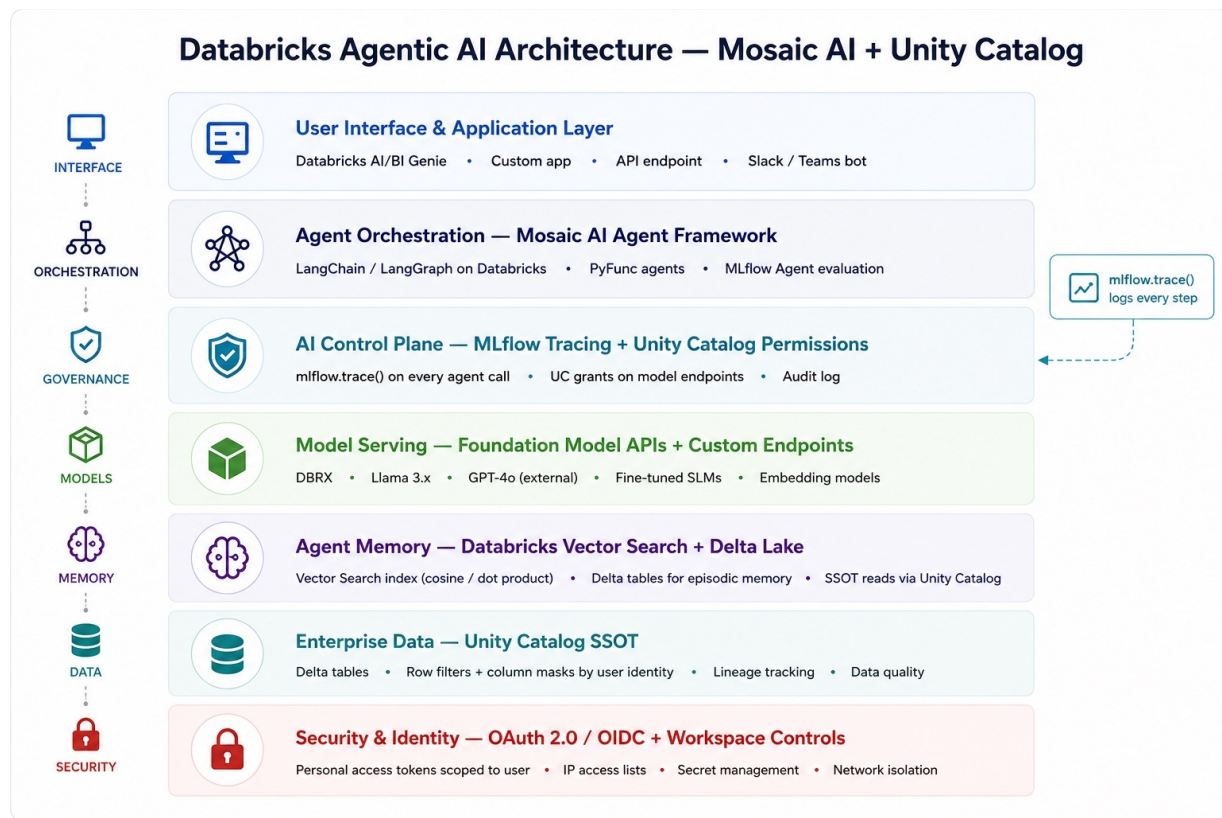
Figure 8.5: Databricks Agentic AI Architecture — Mosaic AI + Unity Catalog. A unified seven-layer stack from Security & Identity at the foundation through Enterprise Data, Agent Memory, Model Serving, AI Control Plane, Agent Orchestration, and User Interface. Every agent call is traced via MLflow; Unity Catalog enforces data access based on the calling user's identity.
