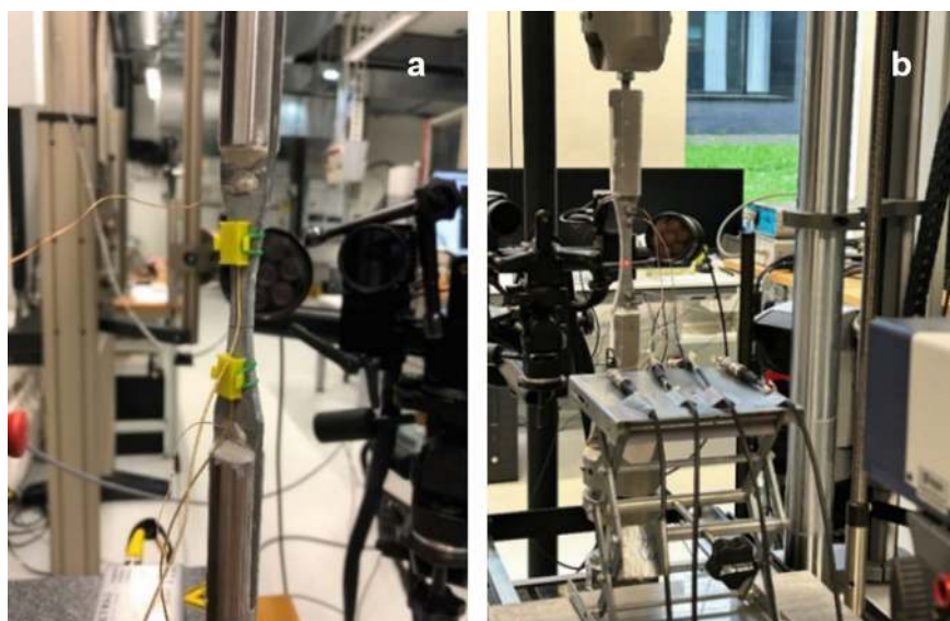
Fig. 4 Static tensile test setup on micro sized specimens
