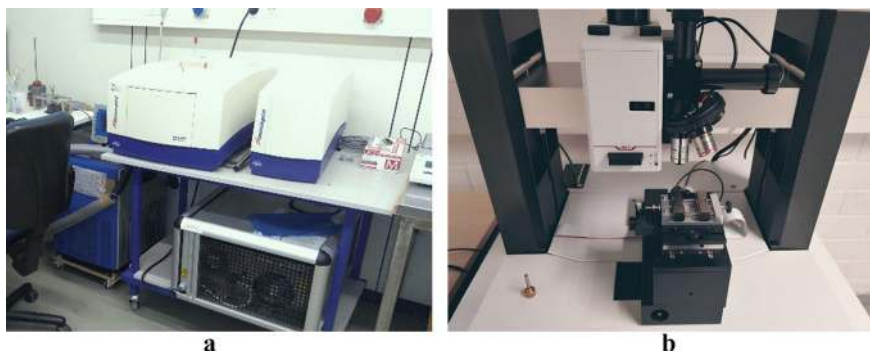
Fig. 2 a Nuclear magnetic resonance measurement equipment and b microindentation set-up
