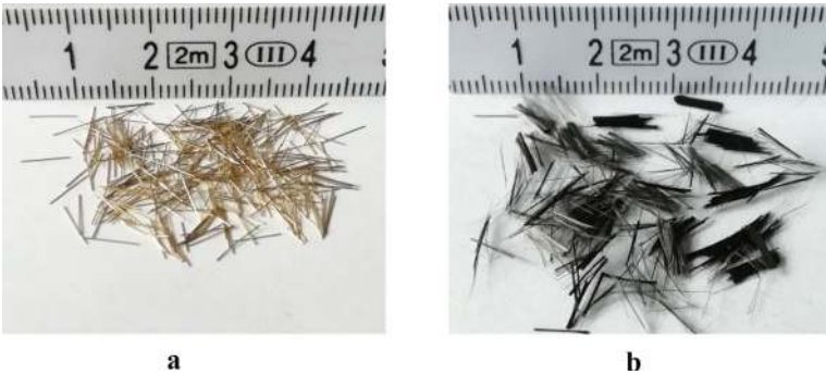
Fig. 1 a Steel fibres, and b carbon fibres (Reproduced from the 20th fib Symposium Proceedings – ReConStruct - Resilient Concrete Structures, held in Christchurch from 11–13 November 2024, article “Influence of different microfibers on the flexural fatigue characteristics of high-strength concrete” page 225—“Fig. 2: steel fibers (left) and carbon fibers (right)” with permission from the International Federation for Structural Concrete (fib) [29])
