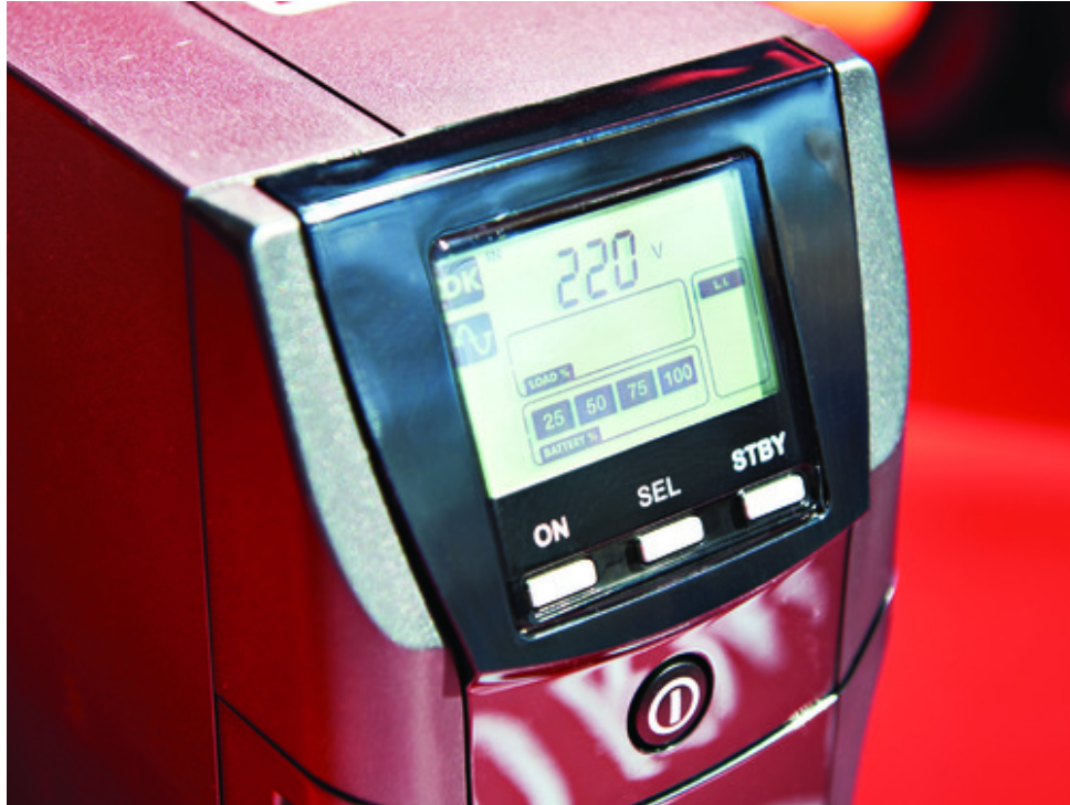
Figure 9.6 Uninterruptible power supply (UPS).
