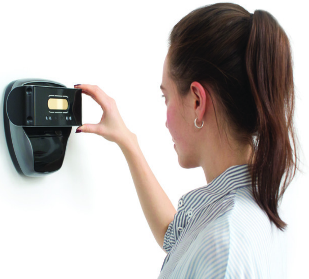
Figure 2.5 Iris scan authentication for entering a facility.
