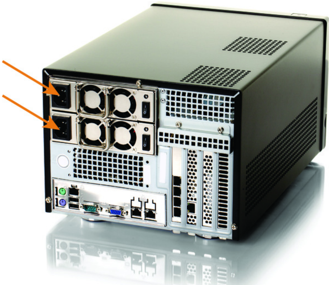
Figure 9.5 Server with dual power supplies.
