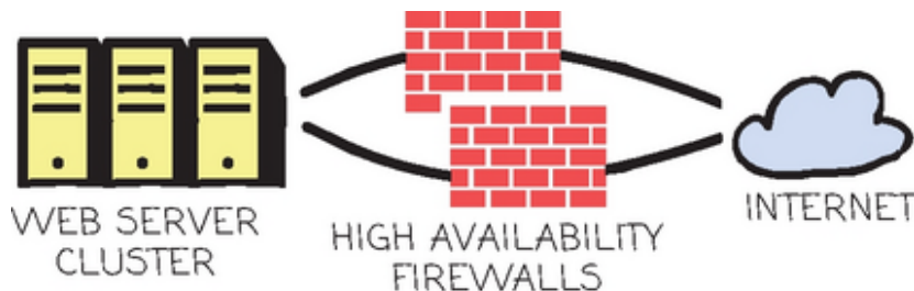
Figure 9.4 Adding redundant network links.
