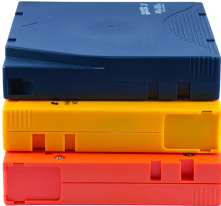
Figure 10.1 LTO backup tapes.
